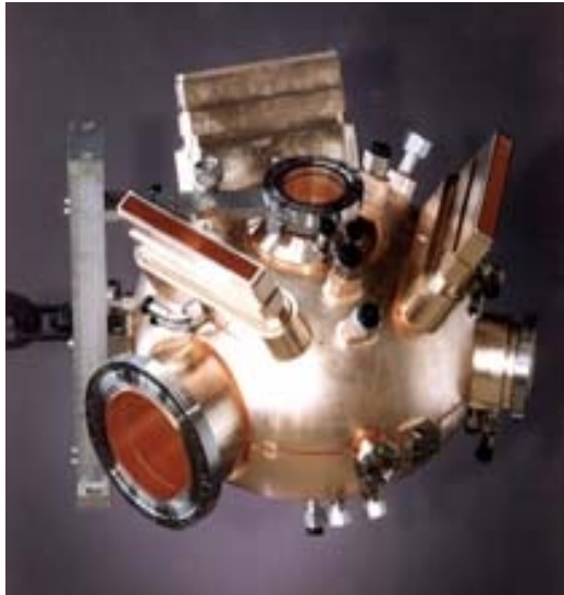
PEP II cavity 476 MHz, single cell, 1 MV gap with 150 kW, strong HOM damping,
