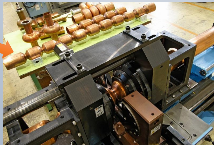
Necking machine at KEK for fabrication of multi-cell seamless cavities
