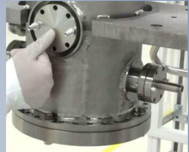
Particle-tight seal with 2 bolts
