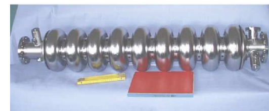
9 cell, 1.3 GHz Nb TESLA cavity
