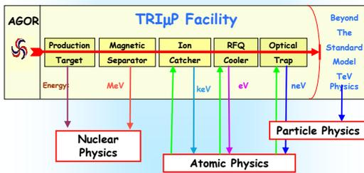
The dual magnetic separator at the TRIμP facility is in operation since mid 2004. It has various operation modes from fragmentation to gas filled mode. Secondary beam can be obtained with high degree of purity.
