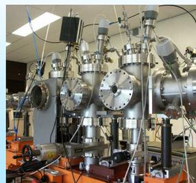
RFQ Radio Frequency Quadrupole cooler, confines and bunches the secondary beam. (being commissioned)
