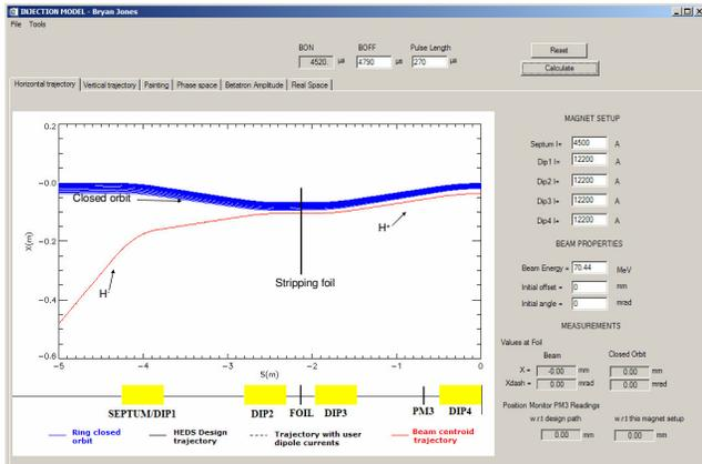
The application allows the user to specify currents for each of the injection dipoles and offsets in position and angle of the injected beam. Trajectories are displayed for the design path and perturbed beam path as well as the closed orbit of the ring. Position and angle of the beam is displayed at the foil and at a position monitor for comparison with experimental data.
