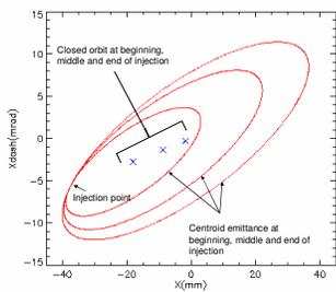
The plots display to the user the status of the accumulated beam at the end of the injection period. It is also possible to view snapshots of the beam at different times of the injection period. The plot left shows three different horizontal closed orbit positions and the beam ellipse associated with each position.
