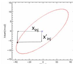
Betatron amplitudes are plotted for comparison with experimental data. Although numerically different, the trend of the betatron amplitude in both planes shows good agreement with measured values.
