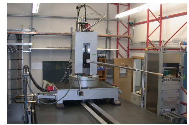
The magnet measuring machine with HALL probe
