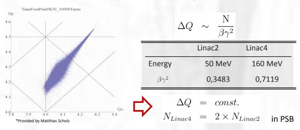
The tune, Q, indicates the number of betatron oscillations pro circulation. Since tune resonances lead to particle losses, the tune shift,  $\Delta Q$ , should be maintained as small as possible. Due to the increasing of the PSB injection energy a doubling of the bunch population becomes feasible while preserving the tune shift.
