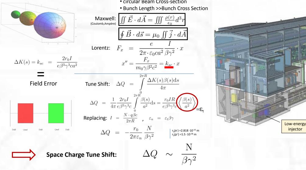
Simple Model: • Charge Distribution is uniform • circular Beam Cross-section
