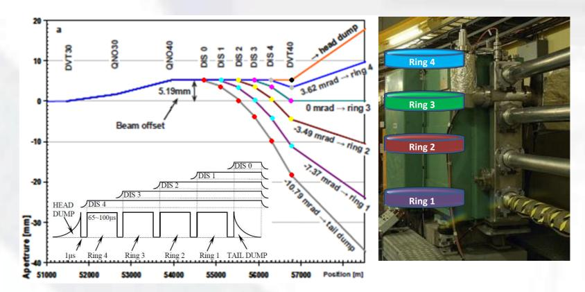
Since the PSBooster consists of 4 Rings the bunch sequences from Linac4 has to be separated into the 4 rings. This is performed by an ensemble of 5 fast ramping kicker magnets. For the reduction of the particle losses during ramping defined chains of bunches are generated by the chopper section of Linac4.
