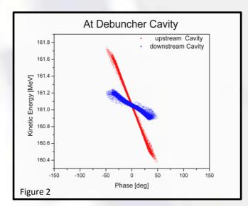
Due to the low energy the energy spread causes a longitudinal expension of the beam. Particles with energy above the average energy are faster and reach the debuncher cavity earlier in time, i.e. later in phase (fig.2). This leads to the generation of an energy shirp. As the synchrotron phase is set to 90 deg., this correlated energy spread can be reduced while conserving of the emittance. The energy swing of ±1.2MeV requires the readjustment of the synchrotron phase for each bunch.
