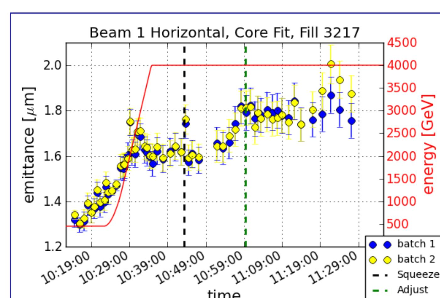
Average emittance of 6 bunches per batch through the LHC cycle for beam 1 horizontal measured with wire scanner, Fill 3217. Batch 1 is colliding at LHCb, batch 2 in ATLAS and CMS.
