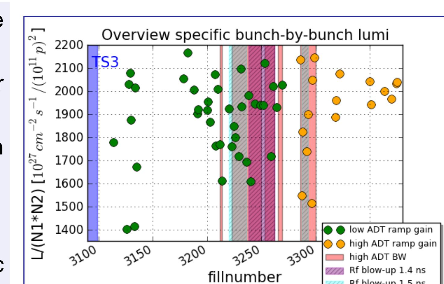
Most-probable average specific bunch-by-bunch luminosity for fills after TS3 in 2012. Measures such as high bandwidth transverse damper (high ADT BW) and RF batch-by-batch blow with target bunch lengths of 1.4 and 1.5 ns are also displayed.
