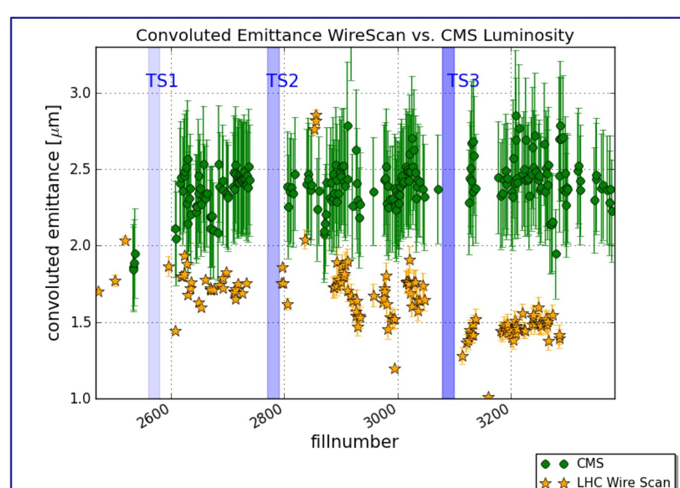
Convoluted, average emittance of the first 144 bunch batch measured with wire scanners at LHC injection (yellow stars) compared to the emittance calculated from CMS peak luminosity (green dots). After Technical Stop (TS) 3: Q20 optics in SPS → smaller emittance at injection, but emittance at collision stayed the same
