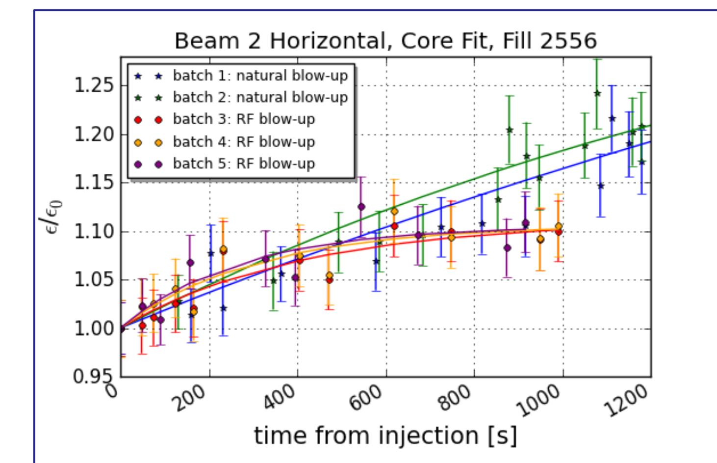
RF batch-by-batch blow-up test with 5 batches of 12 bunches. Batches 1 and 2 are left to natural blow-up. Batches 3, 4 and 5 are longitudinally blown up (target bunch length = 1.6 ns). Relative emittance growth measured with wire scanner (dots) with exponential fit (line).  $\epsilon_0$ : emittance at injection into the LHC.
