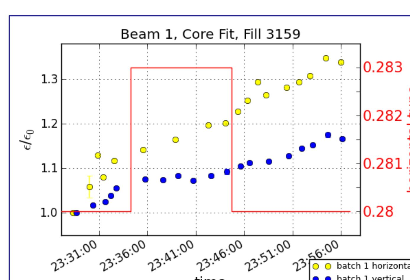
Relative average emittance growth of 6 bunches at injection energy for beam 1 horizontal and vertical measured with wire scanners, Fill 3159.
