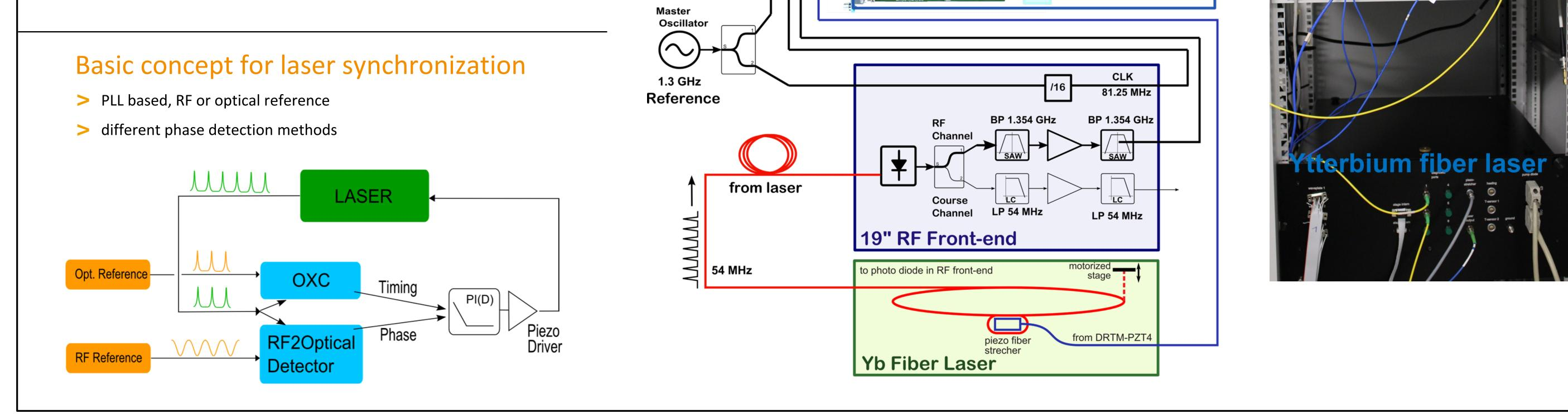
> the analog signal is filtered and amplified by a high voltage power amplifier which drives the piezo stretcher in the laser
