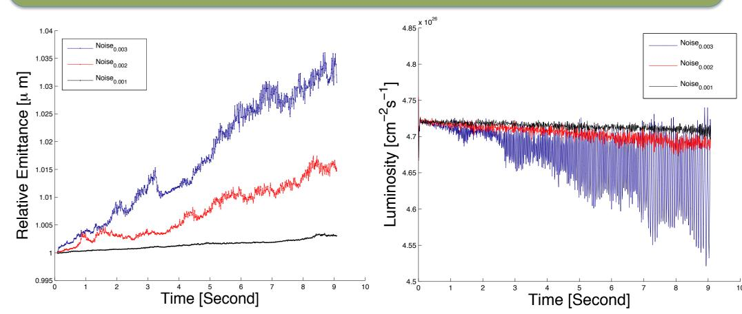
Simulations for round beam profile. Figure on the left shows the relative emittance growth over 100,000 turns. As expected the largest noise that acts on the bunch causes the largest emittance growth. This leads to an increase in bunch size which will lead to a decay in luminosity. As shown in the figure on the right.
