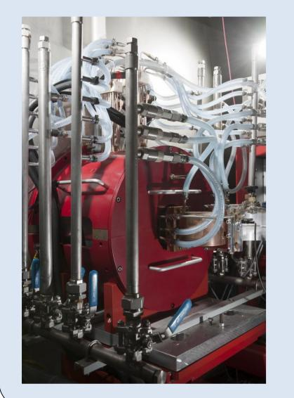
We design, build and operate **electron cyclotron resonance (ECR) ion sources** to produce beams of protons or deuterons with intensities up to ~100 mA.
