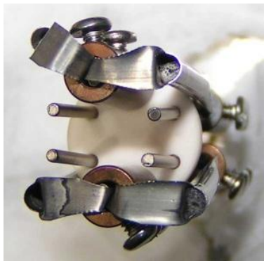
Multi-alkali cathode fabrication
