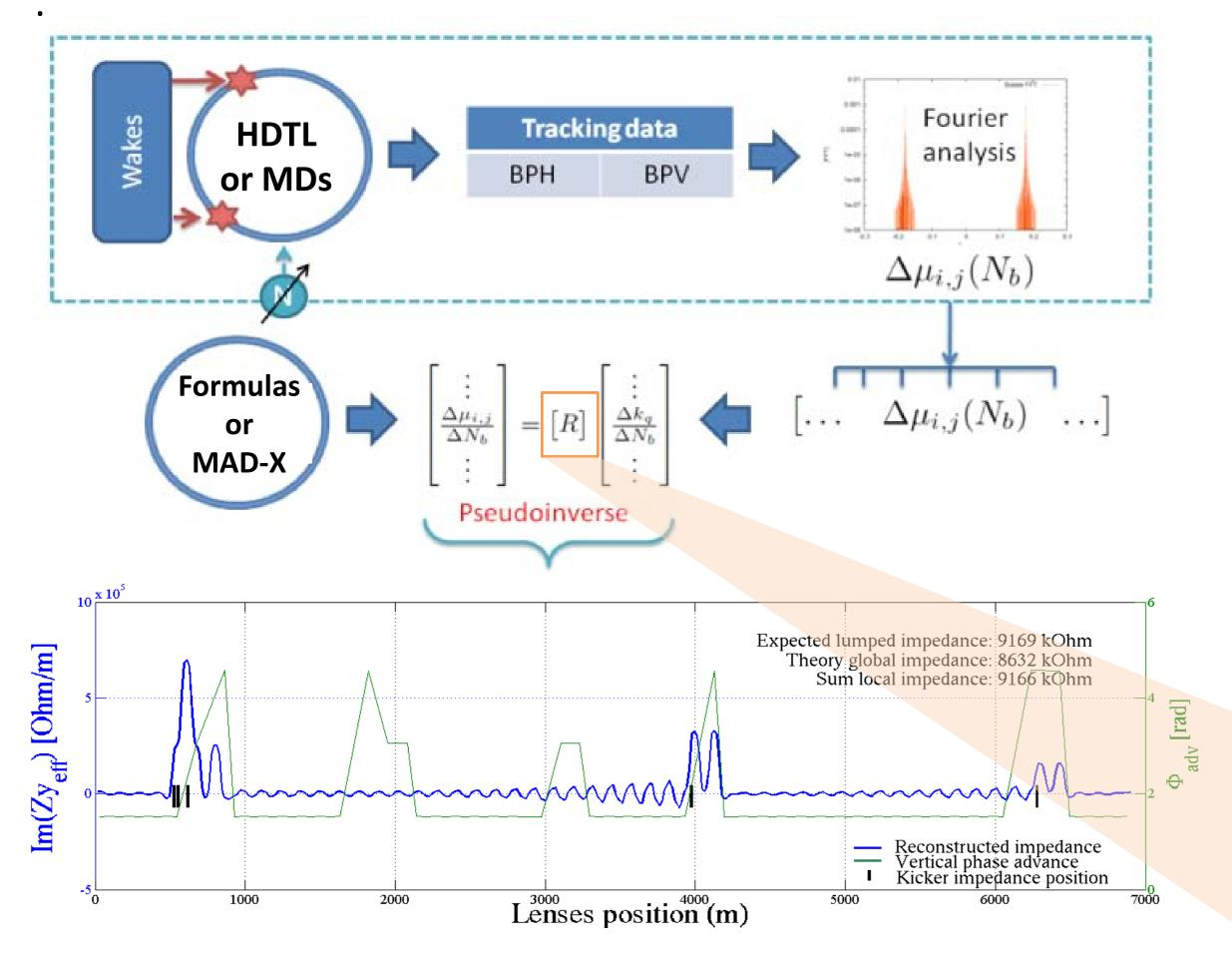
In the limit in which the impedance detuning can be associated with a thin quadrupole detuning, a series of thin lenses can be used to reconstruct the effect of an impedance. Varying the strength of the equivalent lens with intensity we get a quantity proportional to the effective impedance in the place of the lens. A response matrix (to the lens kick) can be constructed either with analytical formulas [6] for the phase advance beating between BPMs or with MAD-X [7]. Vertical plane "R" matrix
