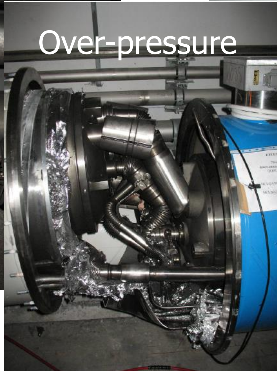
Arcing in an interconnection
