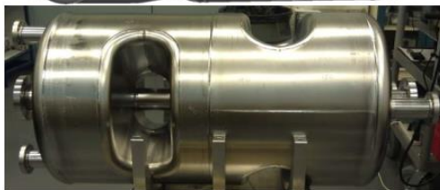
500 MHz, \beta_0 = 1 Double-Spoke Cavity
