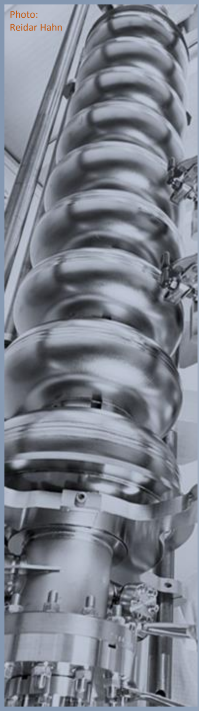
RFD – multi-cell – 953MHz – ODU
