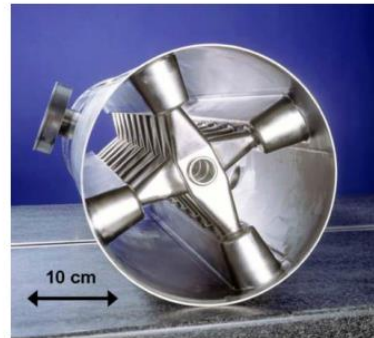
IAP 360 MHz, \beta_0 \sim 0.1 19 gap CH resonator
