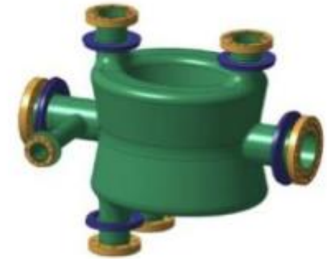
double quarter wave (DQW) – 400MHz – BNL/CERN
