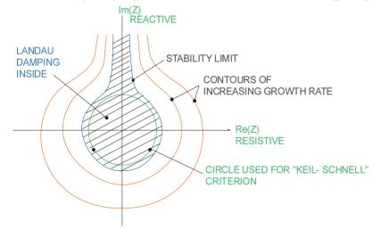
The form of the "bottle" depends on  $g(\Omega)$ ; for most distributions, a circle can be inscribed, giving a handy approximation for the stability limit of un-bunched beams
