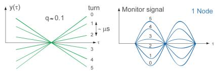
Arrange initial betatron phases so as to have dipole moments up near the head of the bunch down near the tail
