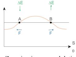
Un-bunched beam in a proton/ion ring Line density  $\lambda(s)$  [particles/m]
