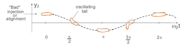
$f = e \frac{Ne}{2} W_1 \delta$   $y_1 = \delta cos \omega_{\beta} t$   $y_2 + \omega_{\beta}^2 y_2 = \frac{f}{m_0 \gamma} = \frac{Ne^2 W_1}{2m_0 \gamma} y_1$   $\Rightarrow y_2 = \delta \left[ cos \omega_{\beta} t + \frac{Ne^2 W_1}{4\omega_{\beta} m_0 \gamma} t sin \omega_{\beta} t \right]$   $tail amplitude y_2 grows linearly with time$
