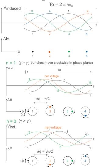
M = 4 bunches, resonator tuned at  $\omega_0$
