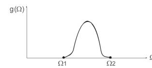
N particles (oscillators), each **resonating** at a frequency between  $\Omega_1$  and  $\Omega_2$  with a density  $g(\Omega)$
