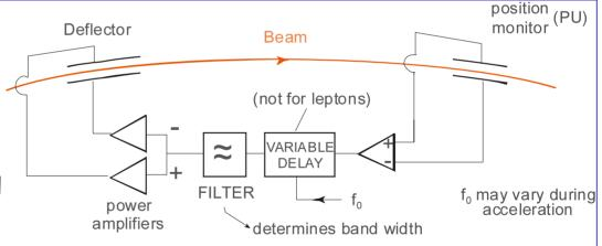
Bandwidth: ~ a few 10 kHz to a few MHz if only resistive wall
