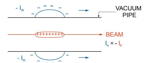
Wall current  $I_w$  due to circulating bunch Vacuum pipe not smooth,  $I_w$  sees an IMPEDANCE (resistive, capacitive, inductive)
