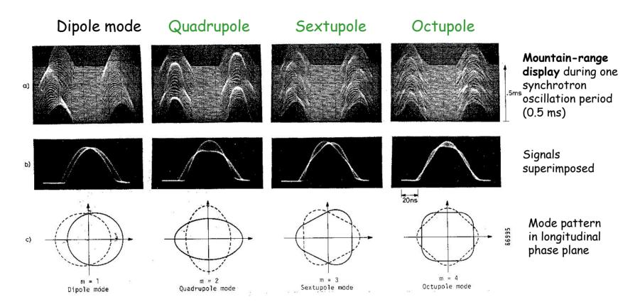
Dipole (m=1) and higher-order (m=2,3,4) modes in a synchrotron with 5 bunches Two adjacent bunches shown. *Note phase shifts between adjacent bunches*
