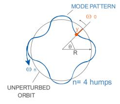
**MODE:** particles are arranged around the synchrotron with a strict correlation between transverse particle positions.
