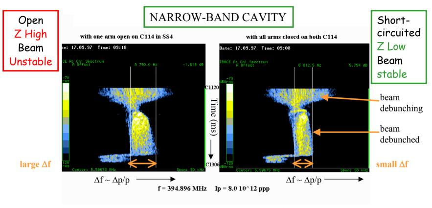
Increase in  $\Delta p/p$  due to coasting beam longitudinal instability in the CERN PS during debunching of protons.
