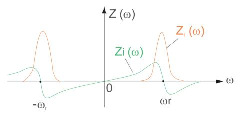
$$Z(\omega) \approx R_s \frac{1 - i2Q \frac{\Delta \omega}{\omega_r}}{1 + \left(2Q \frac{\Delta \omega}{\omega_r}\right)^2}$$
