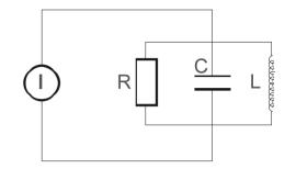
$$\ddot{V} + \frac{\omega_r}{Q} \dot{V} + \omega_r^2 V = \omega_r \frac{R}{Q} \dot{I}$$
