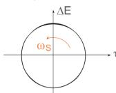
All particles perform synchrotron oscillations – their energy changes with frequency  $\omega_s$
