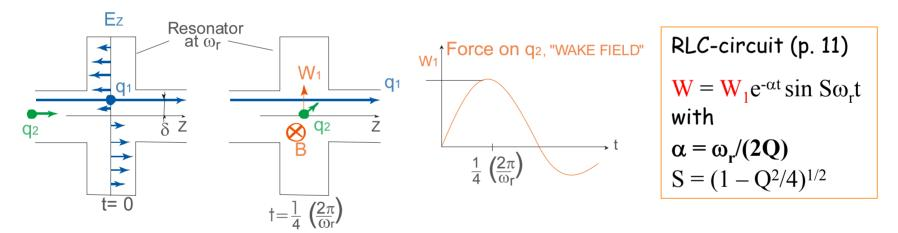
The Wake Field concept is very useful for impedances with short memory where the fields do not act on subsequent bunches but only on particles within the same bunch (single-bunch effects). Example: broad-band impedance (low-Q resonator)
