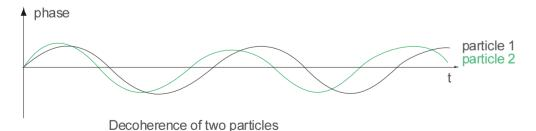
In real machines the beam features a **frequency spread**, so individual particles **move with different speeds** around the ring → the **coherent motion becomes confused** and may **collapse faster** than the **rise time of** the **instability**
