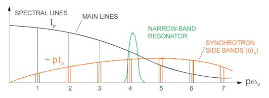
Spectrum of a single bunch performing small-amplitude synchrotron oscillations
