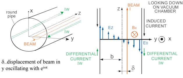
To sustain the differential wall current  $I_w$  a longitudinal electric field  $E_z$  varying across the aperture is required
