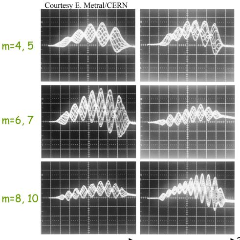
A single bunch with ~10<sup>12</sup> protons and ~150 ns length on the 1.4 GeV injection plateau in the CERN PS (below transition energy)
