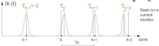
A single bunch performing synchrotron oscillations around a synchronous phase or time
