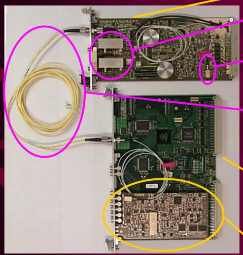
Very Front-End WBTN Card **70MHz Low Pass Filters** Supplied by TRIUMF (Canada) 1310nm Diode Laser Transmitter Tunnel Single-Mode Fibre-Optic Link Surface VME based **Digital Acquisition Board TRIUMF** (Canada) (2 x 12bit 40MHz Acq) WBTN Mezzanine Card (10bit digitisation at 40MHz)
