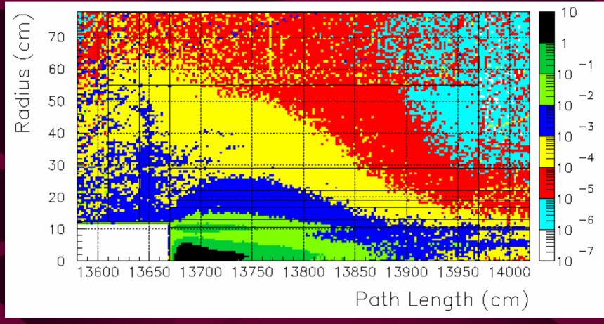
• Peak power density of 1-10 W.kg<sup>-1</sup>.m<sup>-1</sup> (location of ionization chamber)
