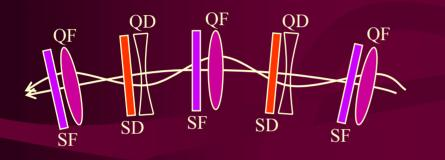
Characteristic Frequency of the Magnet Lattice Produced by the strength of the Quadrupole magnets
