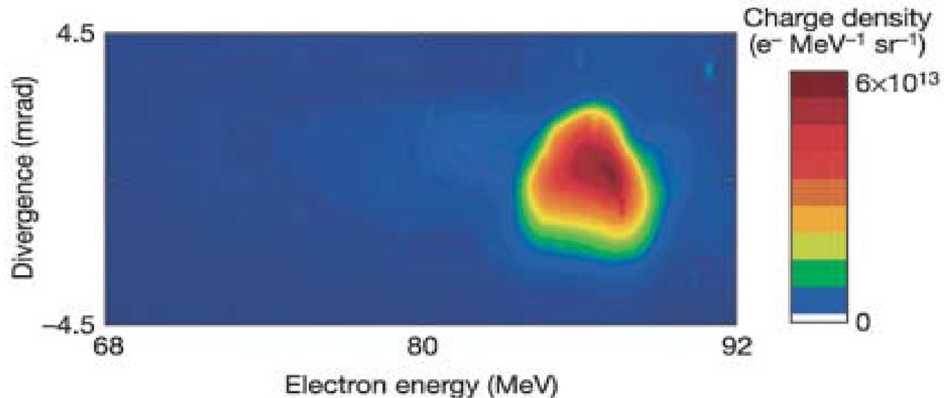
**A laser-plasma accelerator producing monoenergetic electron beams**
