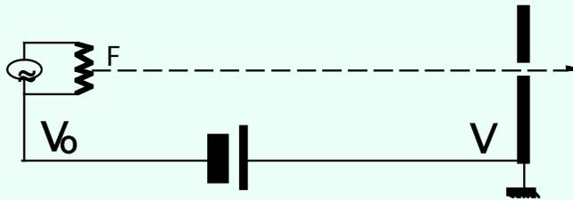
The particle kinetic energy gain is  $\Delta T = q \Delta V$
