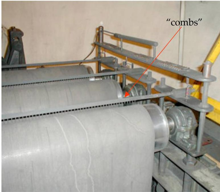
Pelletron Chain from NEC
