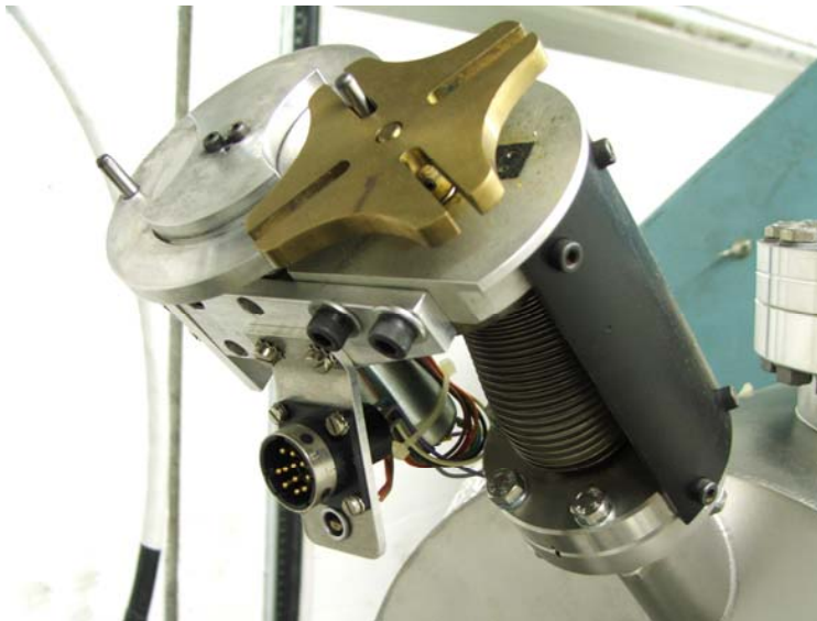
Rotary mechanism driven by electric motor
