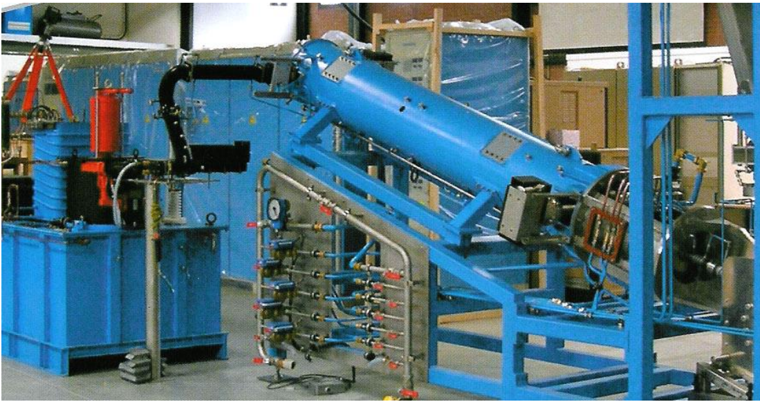
Linear accelerator: 10 MeV, 15 kW L3 Communications, USA
