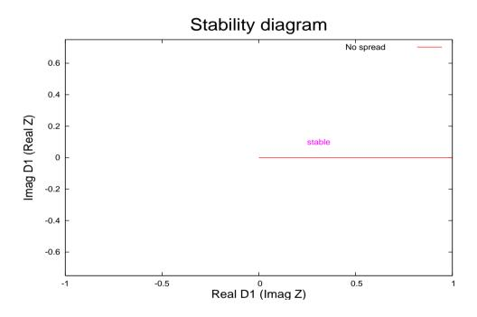
$Real(D_1)$  versus  $Imag(D_1)$  unbunched beam without spread
