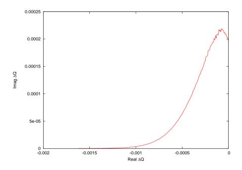
> Stabilization with octupoles, increased strengths
