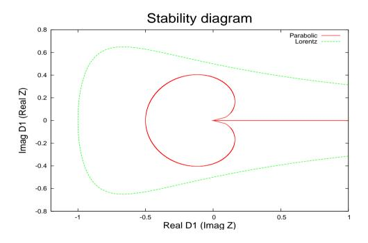
$\mathsf{Real}(D_1)$  versus  $\mathsf{Imag}(D_1)$  for parabolic and Lorentz distribution  $\rho(\omega)$  and unbunched beam
