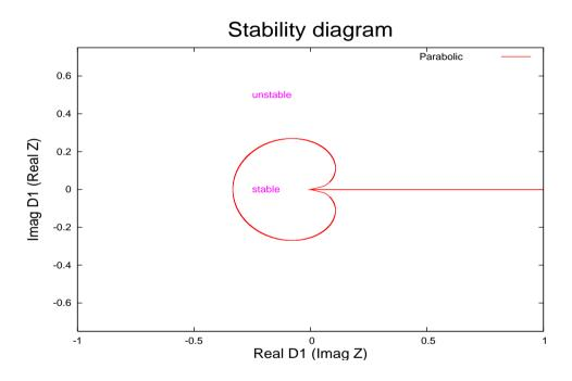
$\mathsf{Real}(D_1)$  versus  $\mathsf{Imag}(D_1)$  for parabolic  $\rho(\omega)$  and unbunched beam
