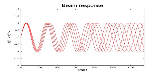
Oscillation of particles with different tunes
