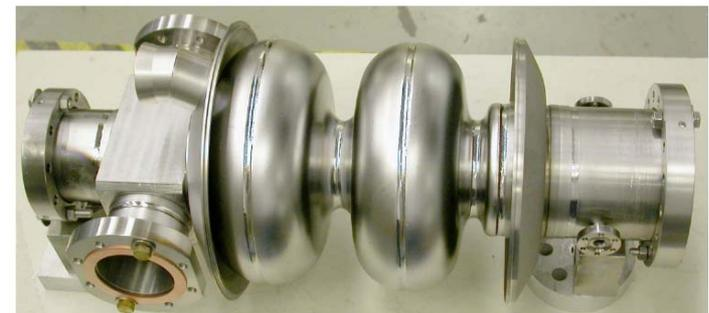
1.3 GHz, 2-cell cavity for Cornell ERL injector.
