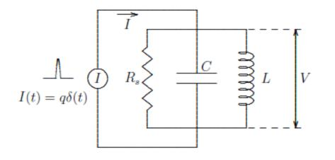
A voltage induced by a charge q at t=0 changes the energy of a second charge q' traversing the cavity at t by U=-q'V(t)=-qq'G(t)
