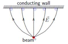
• In fact, to compute the field, one has to introduce an image charge  $(-\lambda)$  at a distance h from the beam:
