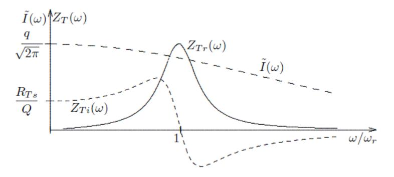
Here again, perform convolution between bunch spectrum and impedance
