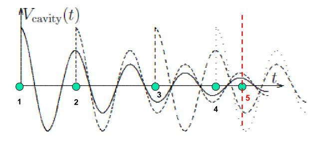
• Effect on particle 5 is the sum of the wakes (Green's) produced by all the particles in front of it.
