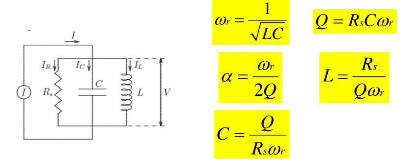
Driving this circuit with a current I gives the voltages and currents across the elements
