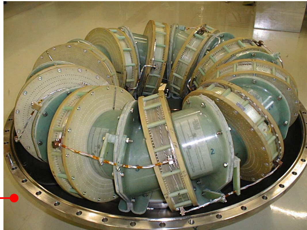
Toroidal magnet of 200 kJ / 160 kW energy store ( B = 4 \text{ T} , dia. = 1.1 m)
