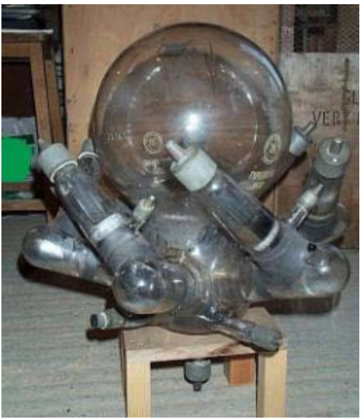
This is a 6-phase device, 150A rating with grid control. It measures 600mm high by 530mm diameter.
