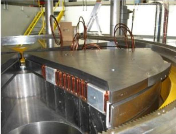
Coils around the pole produce a 'quadrupole-like' field distribution. Field is pushed from low radius to high radius or vice-versa, by changing the sign of the coil current
