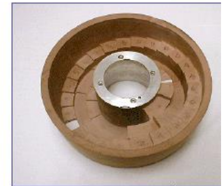
IBA design (3 tracks on single wheel, gating used to adjust modulation)
