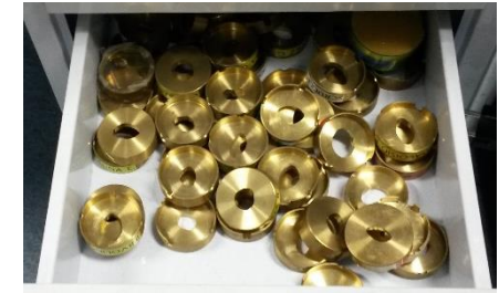
Final collimators and compensators are patient specific
