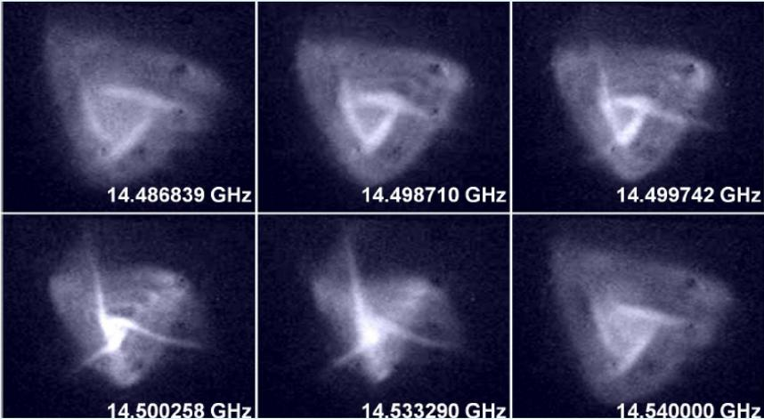
Near axis density depletion takes place because of low EM field. **Most of the resonant modes at  $f > 10$  GHz exhibit holes in near axis zone**
