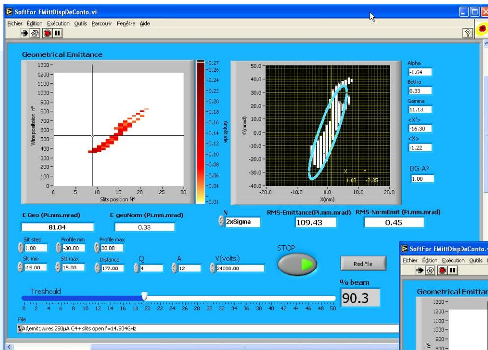
The emittance for the above case was good,  $0.52\pi$  for 100% and  $0.45\pi$  for 90% of the beam.
