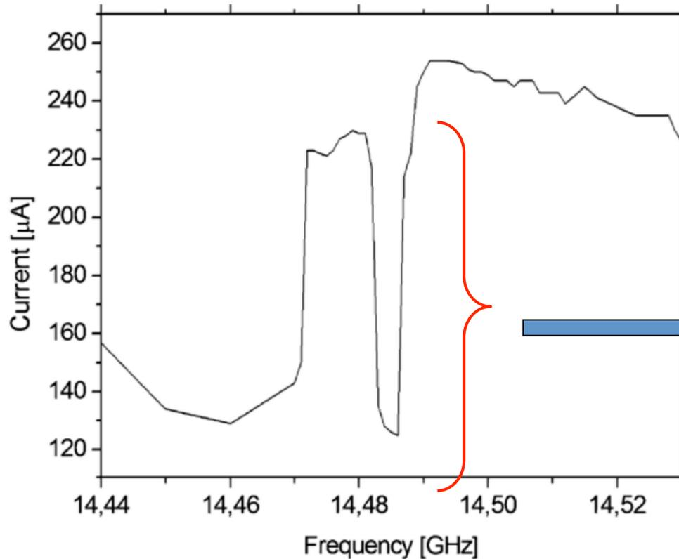
*Trend of the analyzed  $C^{4+}$  current versus the RF frequency.*
