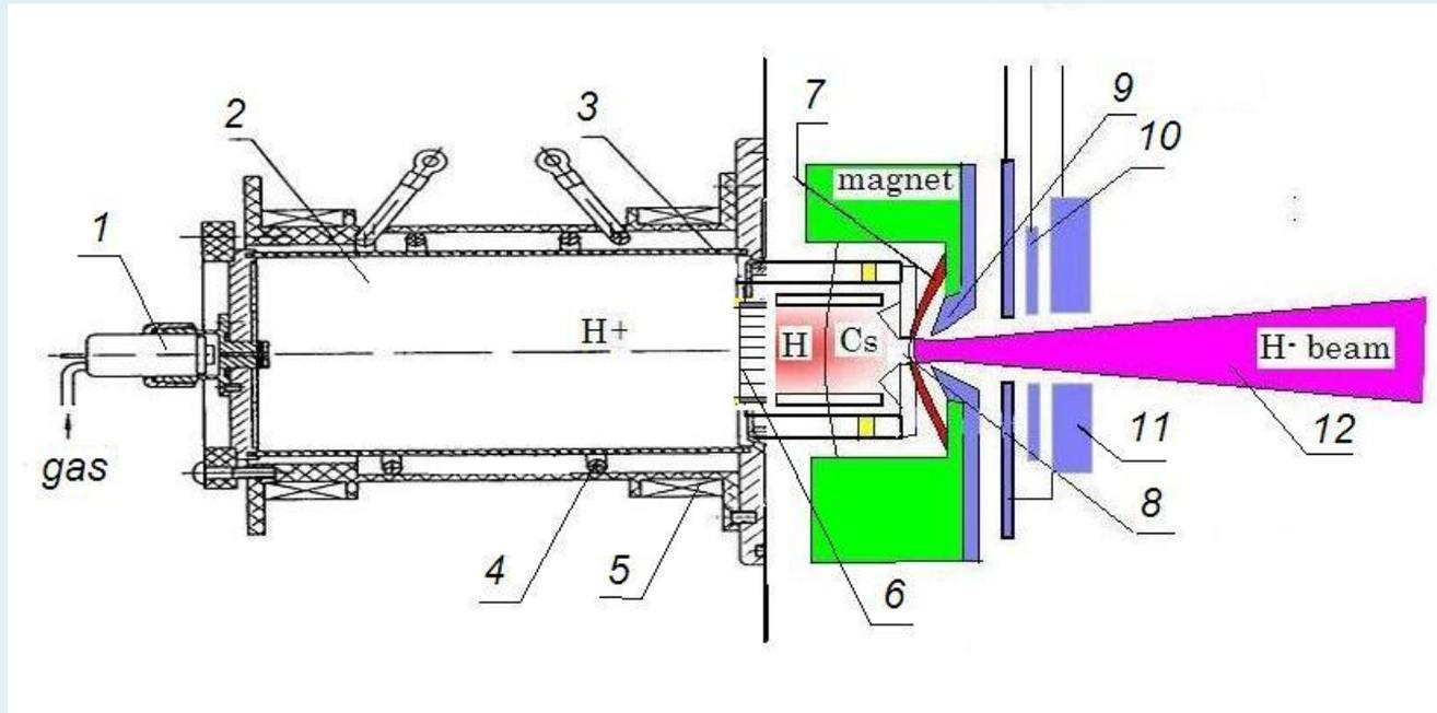
1- gas valve; 2- discharge volume; 3- discharge vessel; 4- helicon saddle like antenna; 5- magnetic coil; 6- ion/atom converter; 7- electron flux; 8- emission aperture (slit); 9- extraction electrode; 10- suppression /steering electrode; 11- ion beam.
