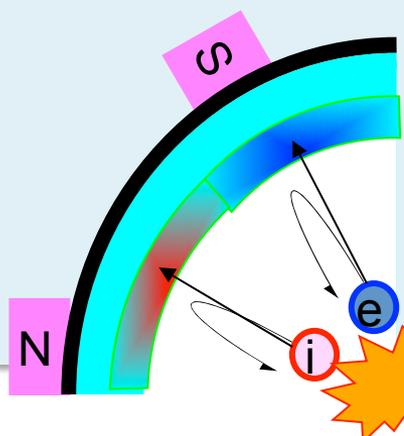
Positive and negative potential formed by **positive charge-up of ion's** and **negative charge-up of electron's** flux repel ions and electrons, thus the plasma confinement is improved.
