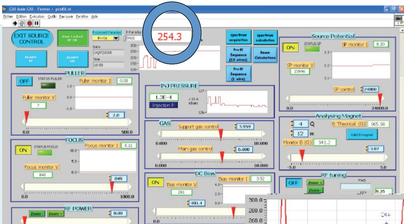
For  $C^{4+}$  the current provided by SuperNanogan was increased from  $200 \mu A$  to  $250 \mu A$  thanks to the frequency tuning (even better improvements obtained with  $H_3^+$ )
