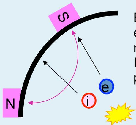
Electrons mainly escape toward to the magnetic field line. Ions also escape to the perpendicular direction.
