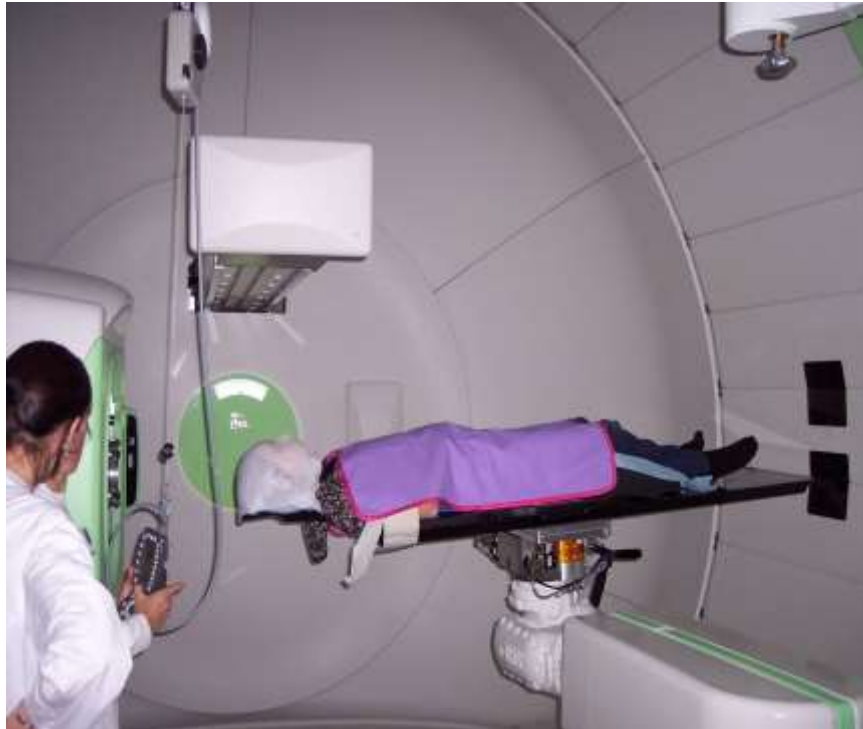
Robot Forte Isocentric motion ( \pm 0.5 mm ) inside treatment volume 6 DOF : pitch & roll ( \pm 15^\circ )
