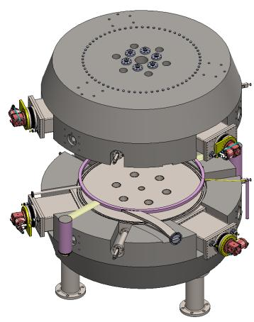
2.2m diameter, 1.6m tall, 30 tonnes, dry cryo-cooled, warm median plane- key technology proof-of-concept demonstrations (magnet, RF, high intensity injector) are now in progress
