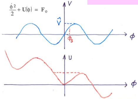
The sum of the potential energy and kinetic energy is constant and by analogy represents the total energy of a non-dissipative system.
