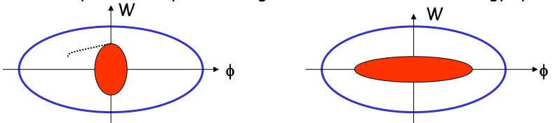
For larger amplitudes, the angular phase space motion is slower (1/8 period shown below) => can lead to filamentation and emittance growth
