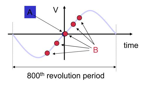
Particle B is performing Synchrotron Oscillations around synchronous particle A.
