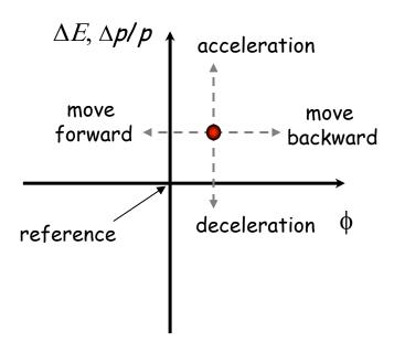
The particle trajectory in the phase space  $(\Delta p/p, \phi)$  describes its longitudinal motion.
