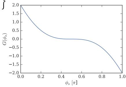
This "RF acceptance" depends strongly on  $\phi_s$  and plays an important role for the capture at injection, and the stored beam lifetime.
