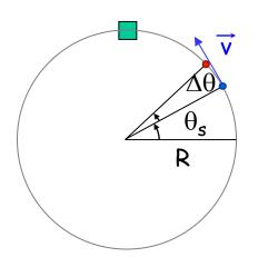
$$f_{RF} = hf_r \implies \Delta \phi = -h\Delta \theta \quad \text{with} \quad \theta = \int \omega \ dt$$
