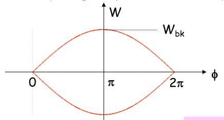
$$W = \frac{\Delta E}{\omega_{rf}} = -\frac{p_s R_s}{h \eta \omega_{rf}} \dot{\varphi}$$
