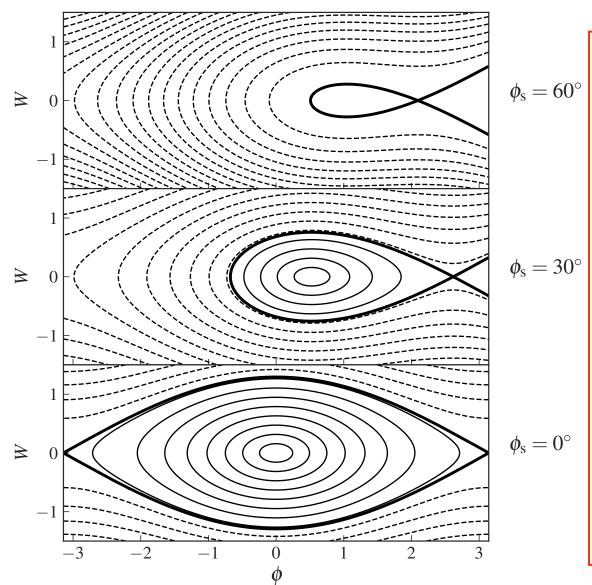
The areas of stable motion (closed trajectories) are called "BUCKET". The number of circulating buckets is equal to "h".
