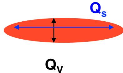
$Q_s$  is the synchrotron tune
