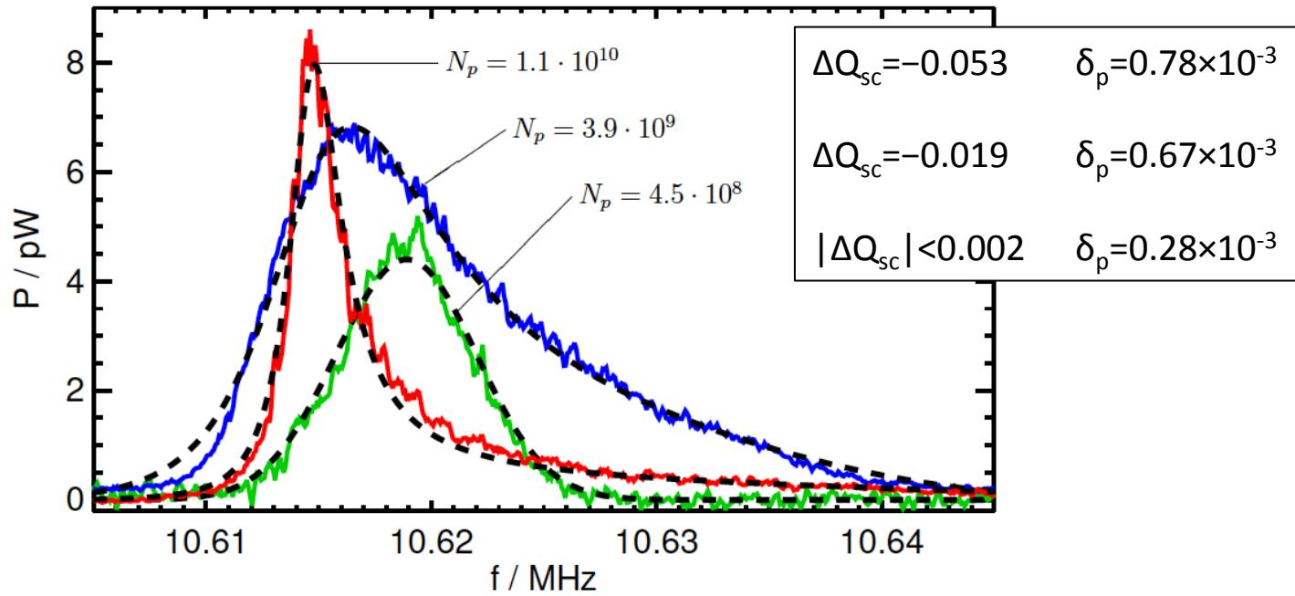
Lower sidebands for  $m=50$ ,  $\text{Ar}^{18+}$  beams in SIS18 at GSI,  $f_0=214$  kHz
