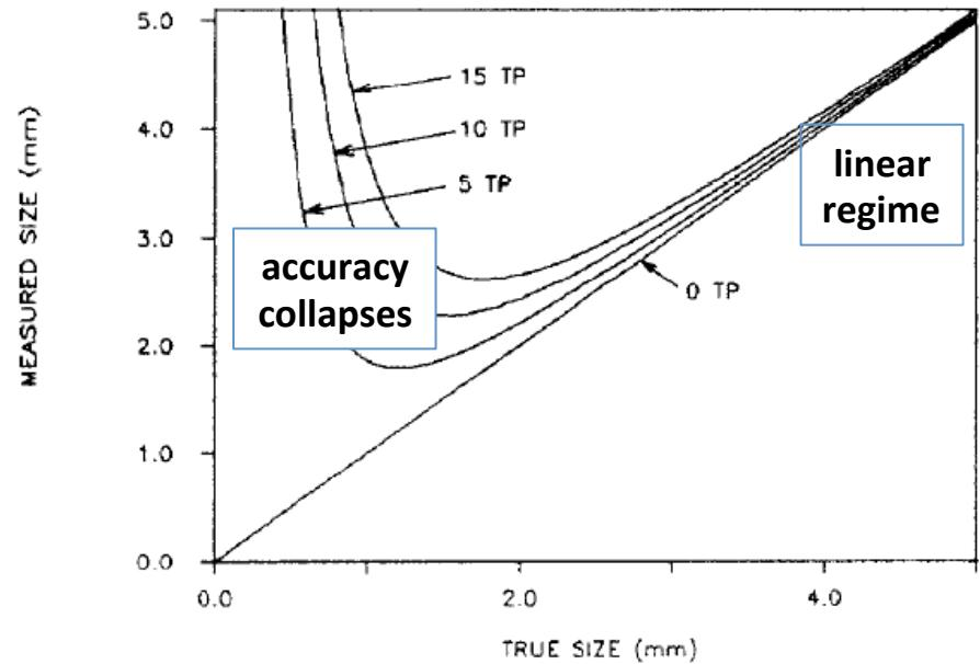
Model for IPM measurements in AGS bunched beams. R.Thern, PAC1987
