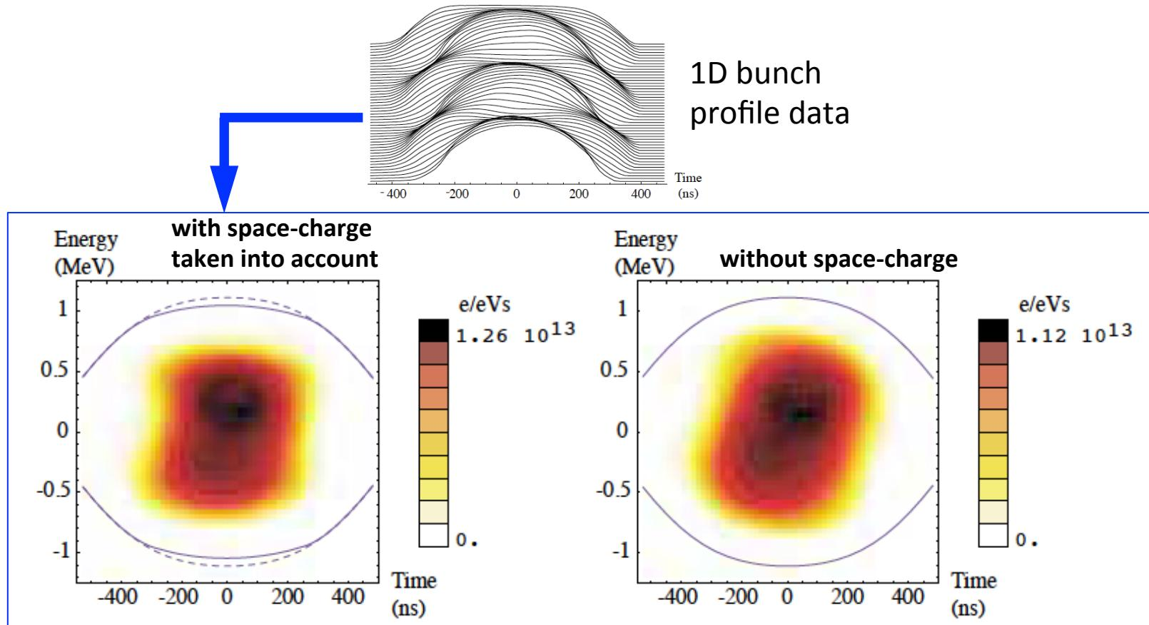
Phase space reconstruction for a CERN PS Booster bunch,  $6.5 \times 10^{12}$  p, 100 MeV
