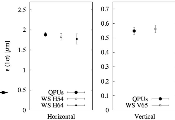
Comparison of the transverse emittance measurements using the quadrupole pickup and the wire scanner in CERN PS,
