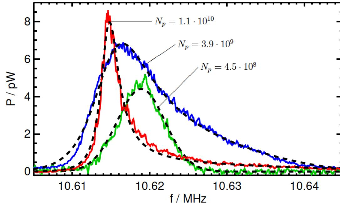
Lower sidebands for  $m=50$ ,  $\text{Ar}^{18+}$  beams in SIS18 at GSI,  $f_0=214$  kHz
