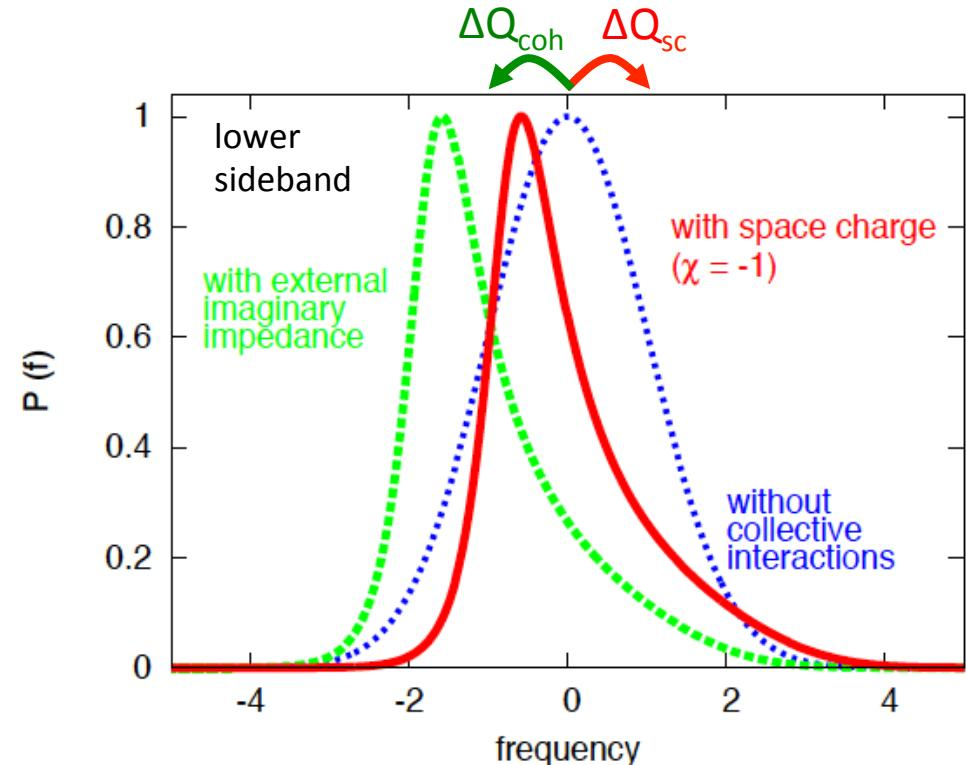
$$\chi = \frac{\Delta Q_{sc}}{\delta Q_\xi} \quad \Delta Q = (\Omega - (m - Q_f)f_0)/f_0 \quad \delta Q_\xi = |m\eta - (Q_f\eta - Q_0\xi)| \delta p/p$$
