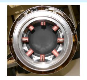
Figure 1: View of the BHM from the dump. The BHM sensors are inside the caps. Four loops of the magnetic-coupled BPM are right in front of the BHM sensors.
