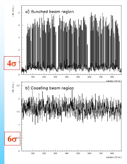
Figure 11.2: The time structure of the proton interaction for an outer target wire at different distances of the wire to the beam center: a) wire  $\approx 4\sigma$  from the beam center and b) wire  $\geq 6\sigma$  from the beam center.
