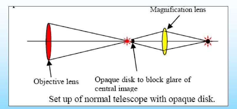
When using OTR or SR (narrow cone) the diffraction fringes makes tail surrounding from the central beam image. Intensity of diffraction tail is in the range of 10<sup>-2</sup> -10<sup>-3</sup> of the peak intensity. The diffraction tail disturb an observation of week object surrounding from bright central beam
