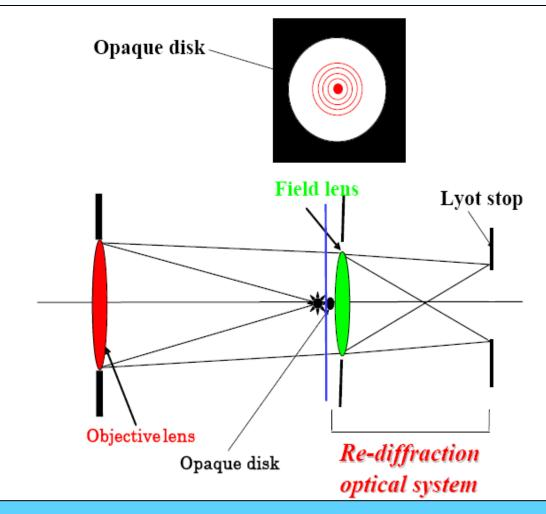
The first lens (objective lens) makes a real image of the object (beam image) on to a blocking opaque disk
