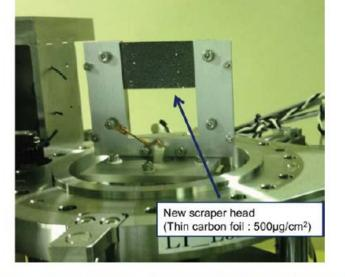
Figure 2: Picture of the new scraper head with the thin carbon foil. The carbon foil is mounted by the metal foil folder.
