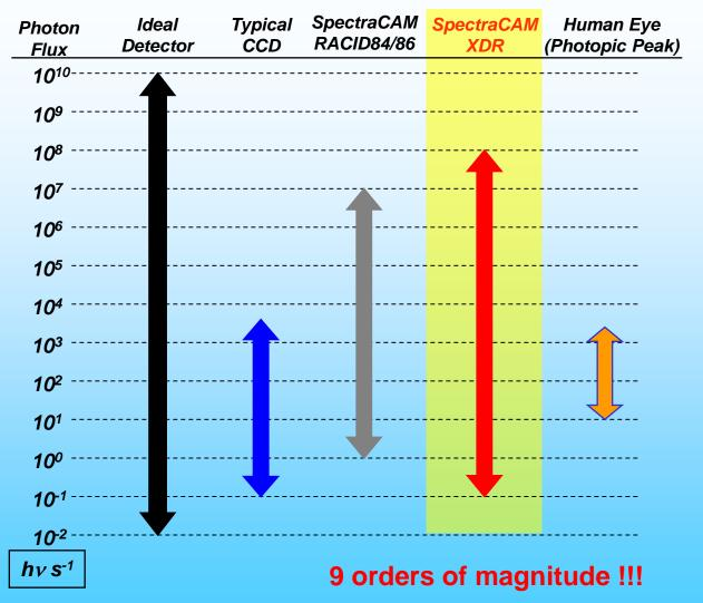
SPECTRACAM XDR: High resolution scientific imaging camera system using Charge Injection Device capable of extremely high dynamic range and random pixel addressing Page 46
