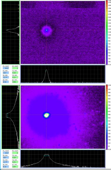
High Dynamic Range Beam Imaging with Two Simultaneously Sampling CCDs; , P. Evtushenko, D. Douglas; IBIC2012, Tsukuba, Japan
