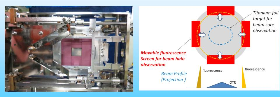
Two-Dimensional and Wide Dynamic Range Profile Monitor Using OTR / Fluorescence Screens for Diagnosing Beam Halo of Intense Proton Beams, Y.Hashimoto et al., HB2014, East Lansing, USA
