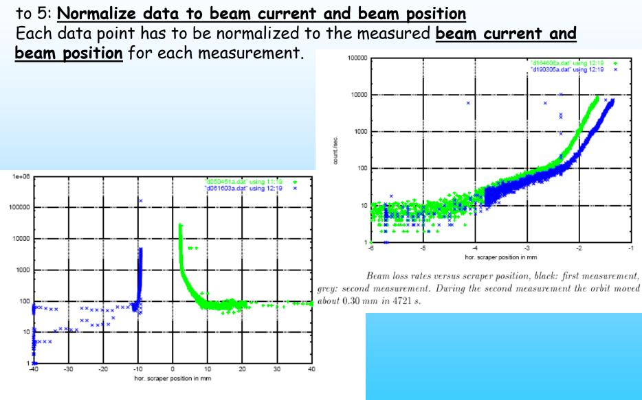
Beam loss rates versus scraper position. The orbit movement causes an artificial asymmetry in the measurement results
