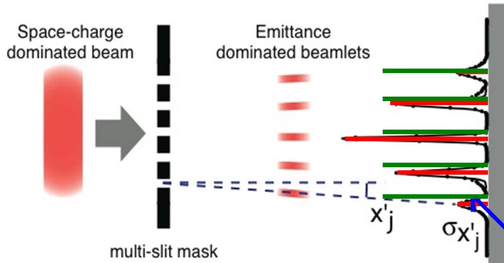
To measure the emittance for a space charge dominated beam the used technique is the well known pepper-pot
