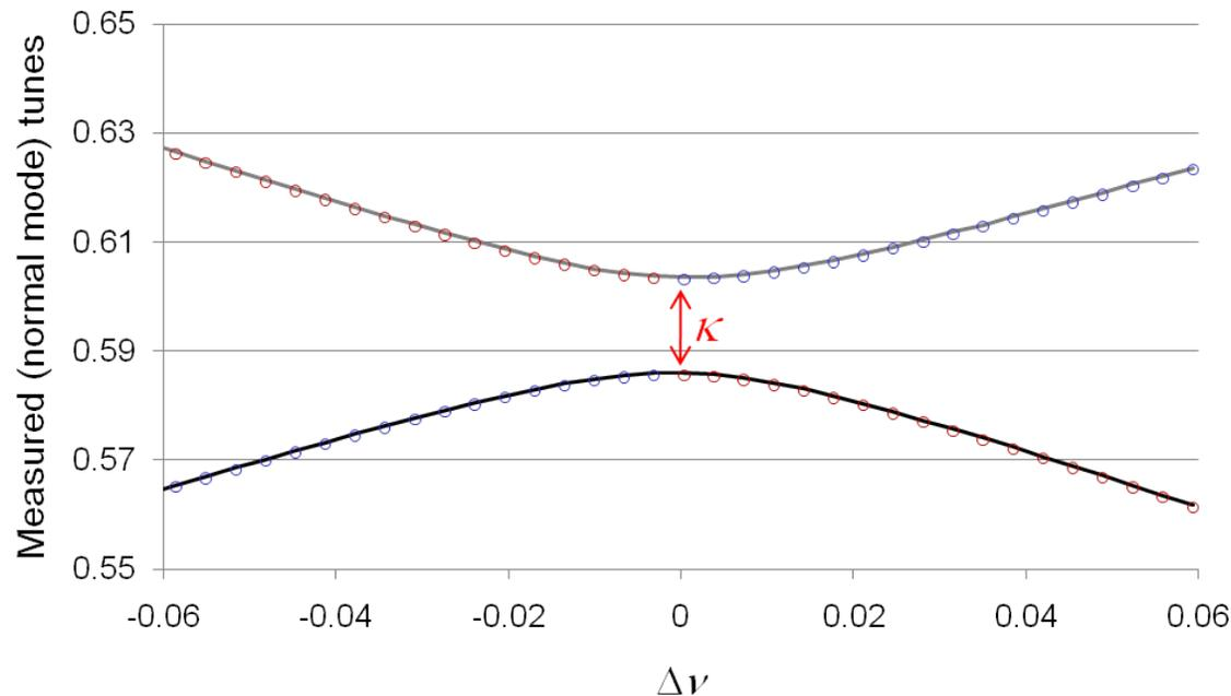
Major sources of coupling in storage rings are quadrupole tilts and sextupole alignment.
