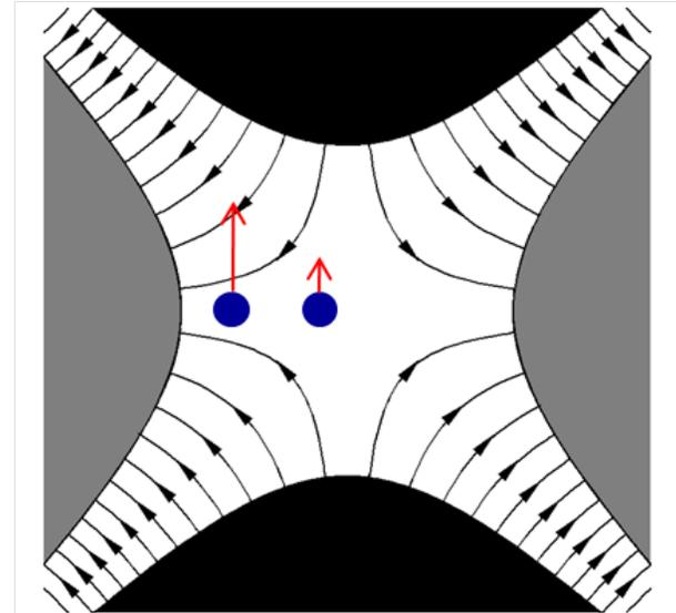
In a storage ring, skew quadrupole fields often arise from quadrupole tilts, and from vertical alignment errors on sextupoles.
