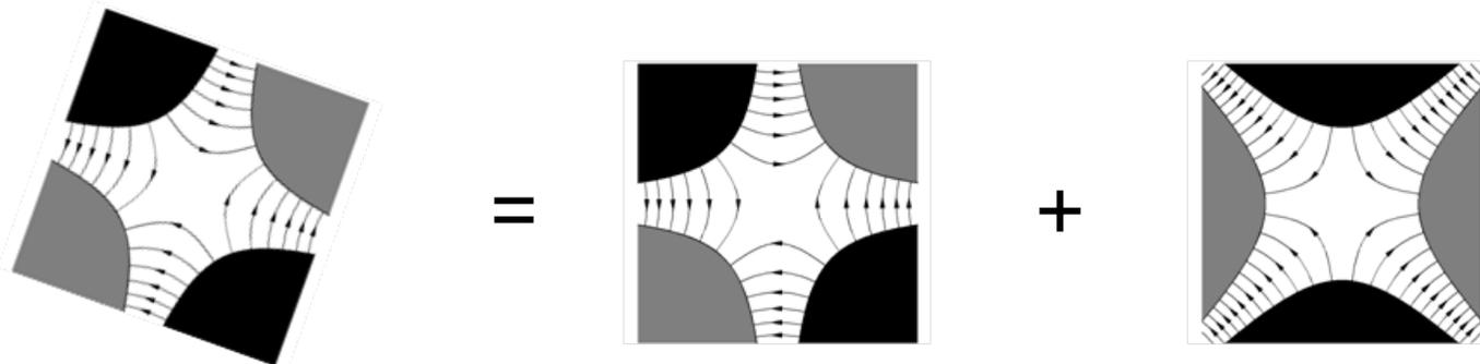
When particles pass through a skew quadrupole, they receive a vertical kick that depends on their horizontal offset. As a result, quantum excitation of the horizontal emittance feeds into the vertical plane.
