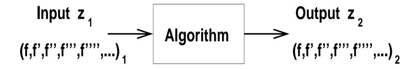
Can extract a truncated Taylor map of a beam line or ring by pushing the identity map f(x) = (a, 1, 0, 0, 0...) through the algorithm as if it is a vector in phase space! The maps are provided with the desired accuracy and to any order.
