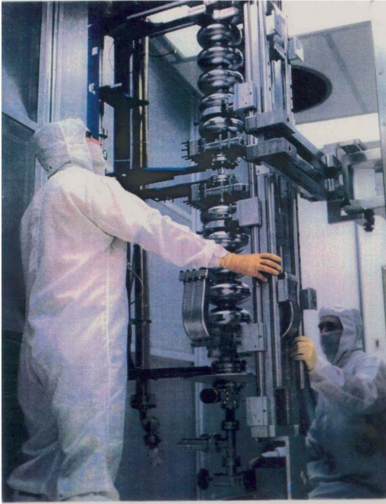
A super-conducting cavity is often a multi-cells assembly. Many such cavities can be put in a single cryostat.
