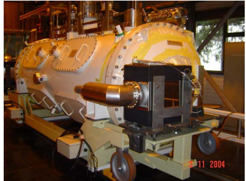
The SC cavity of the synchrotron light source SOLEIL made of two single cells
