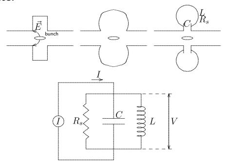
Cavities have narrow band oscillation modes which can drive coupled bunch instabilities. Each resembles an **RCL** - **circuit** and can, in good approximation, be treated as such. This circuit has a shunt impedance  $R_s$ , an inductance L and a capacity C. In a real cavity these parameters cannot easily be separated and we use others which can be measured directly: The **resonance frequency**  $\omega_r$ , the **quality factor** Q and the **damping rate**  $\alpha$ :
