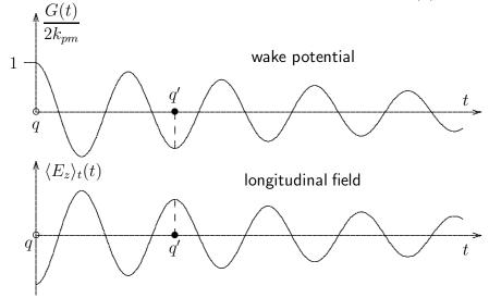
The wake potential is related to the longitudinal field  $E_z$  by a field integration which follows the particle with speed  $v \approx c$  through the object length while taking the momentary field value
