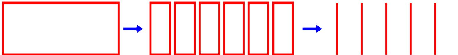
Thick quadrupole  $\Rightarrow$  thin quadrupoles  $\Rightarrow$  "kicks"
