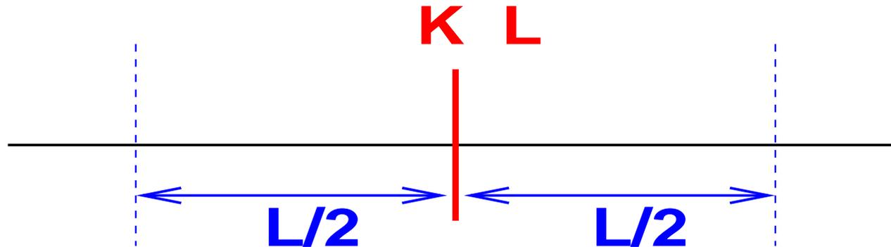
**One thin quadrupole "kick" between two drifts of half length**
