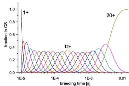
Charge state evolution for  $\text{Ti}^+$ -ions in an EBIT with a current density of  $10^4 \text{ A/cm}^2$  and an electron energy of 5 keV.
