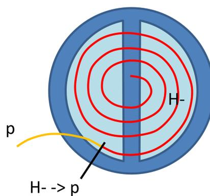
Charge exchange injection (to synchrotron).
