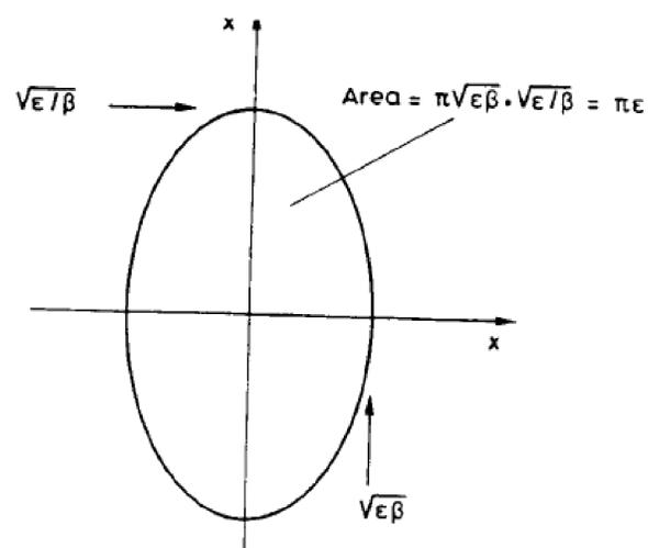
The area within the contour is proportional to the emittance of the beam. At constant energy we express this as the area  $\epsilon = \int y' dy$  in units of  $\pi$ .mm.milliradians. We have shown
