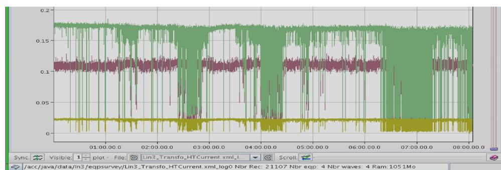
The CERN Linac3 ion source, average beam current per pulse over a period of 8hrs.
