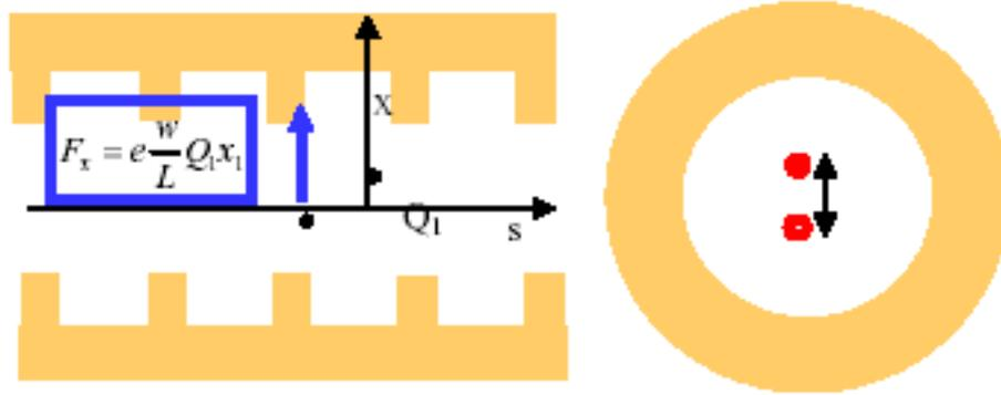
a (source) charge  $Q_1$  traveling with a (small) offset  $x_1$  respect to the center of the RF structure perturbs the accelerating field configuration and leaves a wake field behind. A following (test) particle will experience a transverse field proportional to the displacement and to the charge of the source particle:
