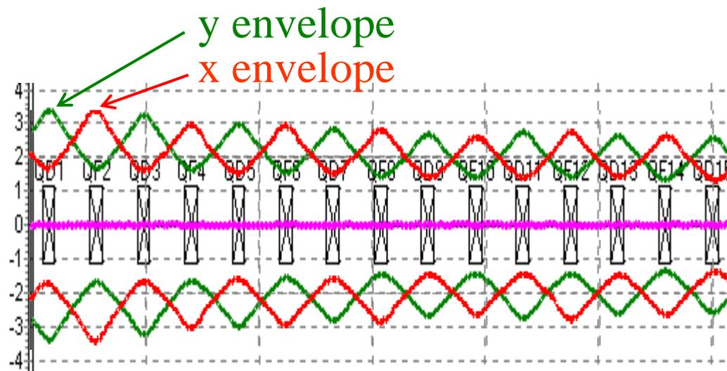
sequence of focusing and defocusing quadrupoles
