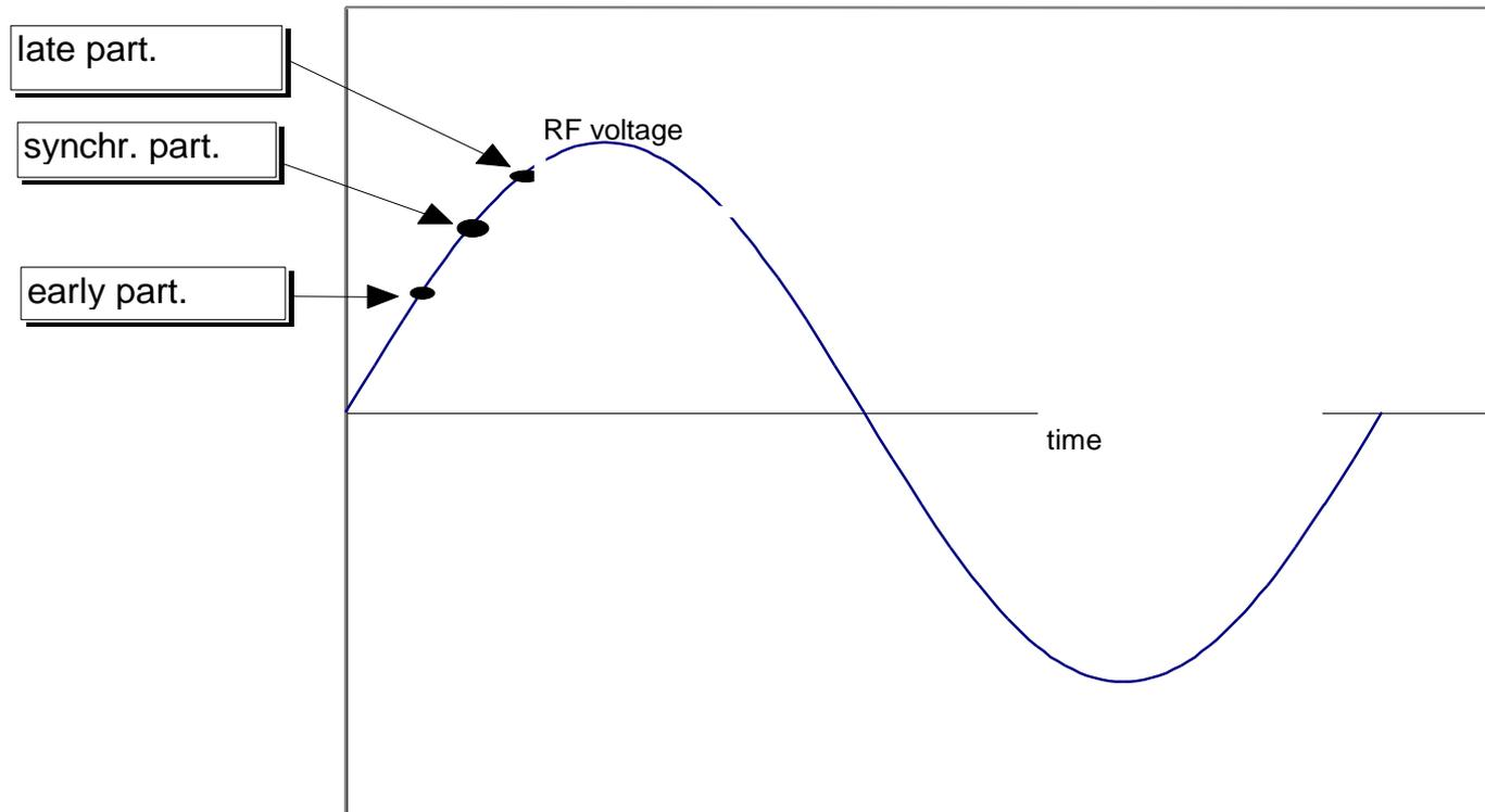
for phase stability we need to accelerate when  $dE_z/dz > 0$  i.e. on the rising part of the RF wave
