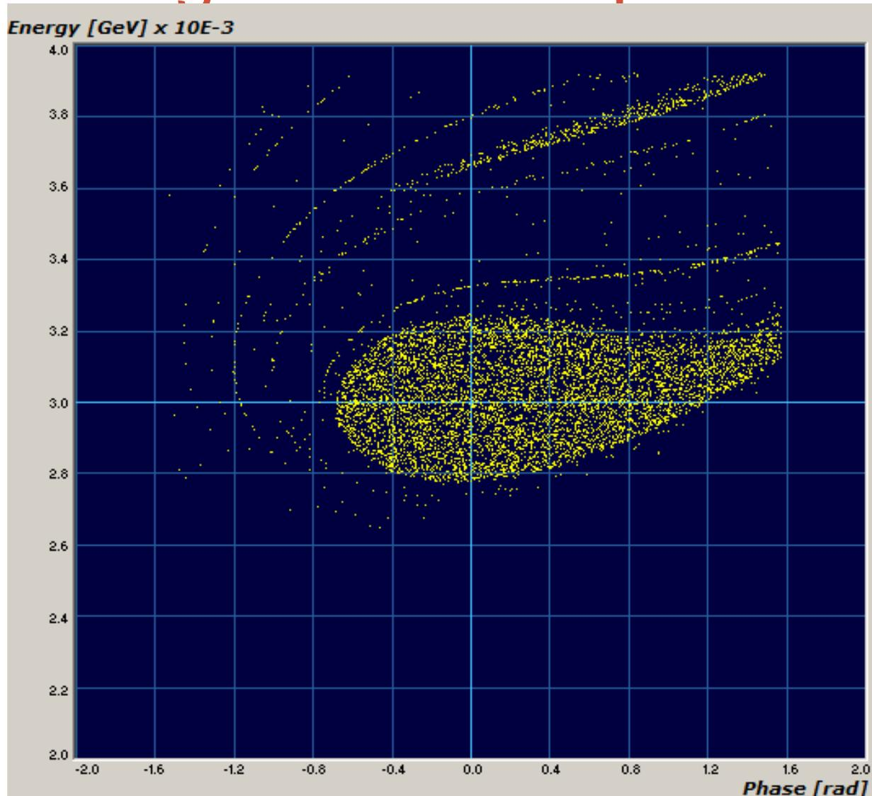
Plot of the longitudinal acceptance of the CERN LINAC4 DTL (352 MHz, 3-50 MeV). Obtained by plotting the survivors of very big beam in long phase space.
