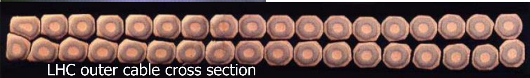
7500 km of superconducting cables with tightly controlled properties (state-of-the-art production)
