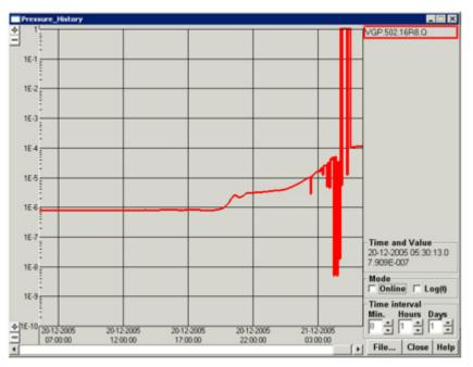
Pressure versus time during the warm up of the LHC helium distribution line
