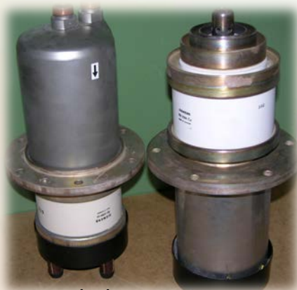
Thales RS 1084 CJ < 30 MHz, 75 kW \eta < 78% (class B)
