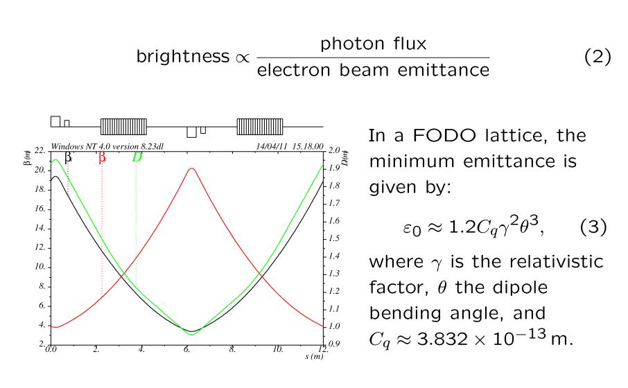
To achieve a natural emittance of 6 nm in a 3 GeV FODO lattice, we need a minimum of 86 dipoles (43 FODO cells).
