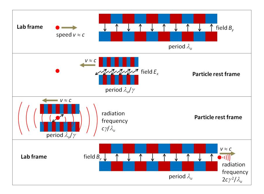
A detailed analysis of the undulator radiation gives the wavelength of the undulator radiation (observed along the axis of the undulator):
