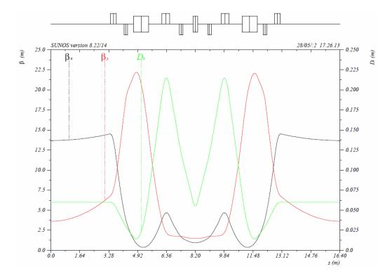
Superbend detuned Triple Bend Achromat (TBA) in the Advanced Light Source. *C. Steier et al, Proceedings of EPAC'02, Paris, France (2002).*  Based on the desire for high brightness, hard x-ray output, we have decided on:
