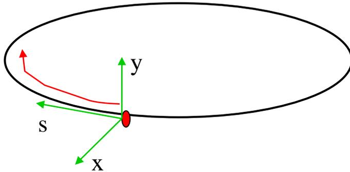
→ choose the longitudinal coordinate as the free parameter for the equations of motion
