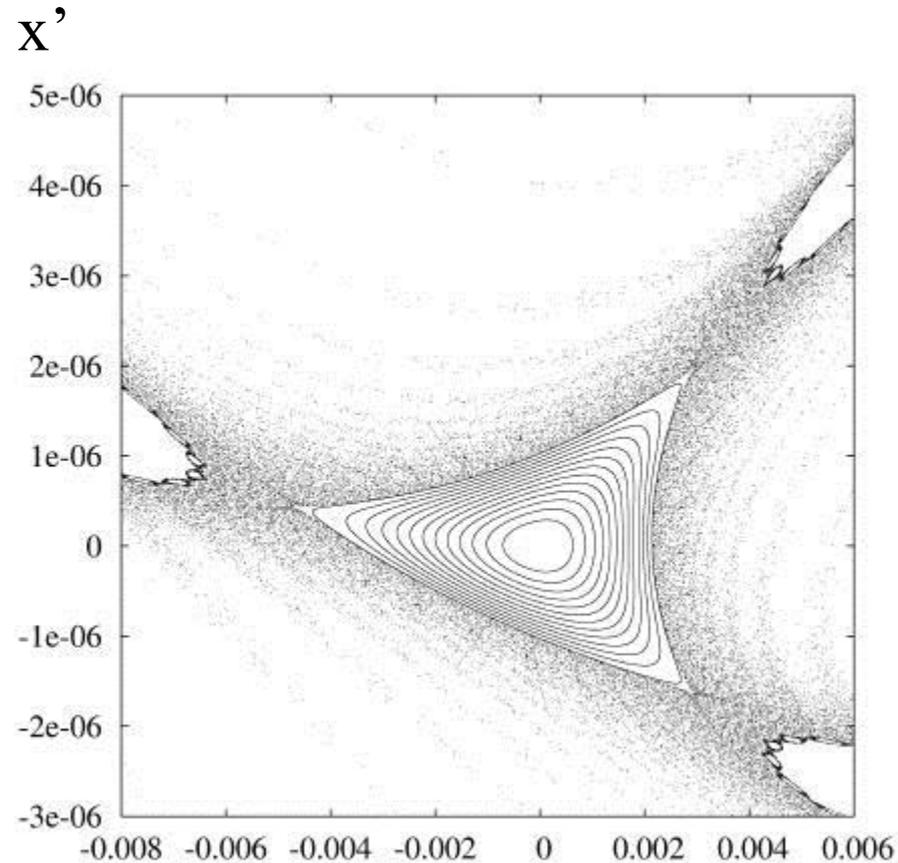
for large amplitudes and near the separatrix the intersections fill areas in the Poincare Section → chaotic motion;
