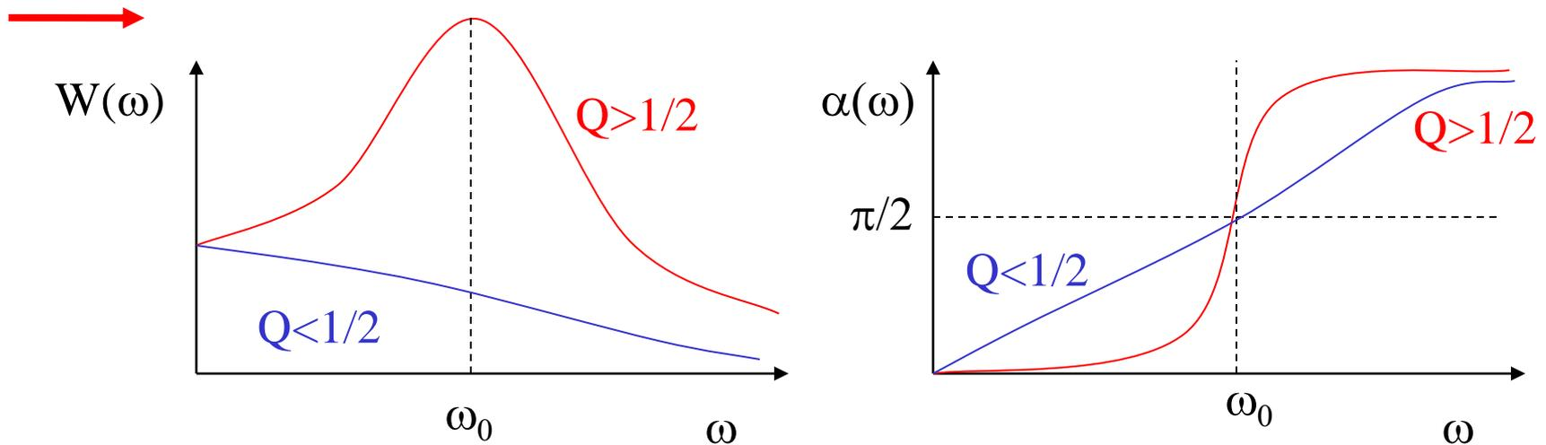
oscillation amplitude can become large for weak damping
