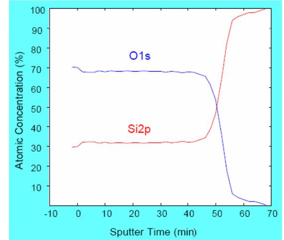
If sputter rate is known, thickness of the surface layers can be calculated.
