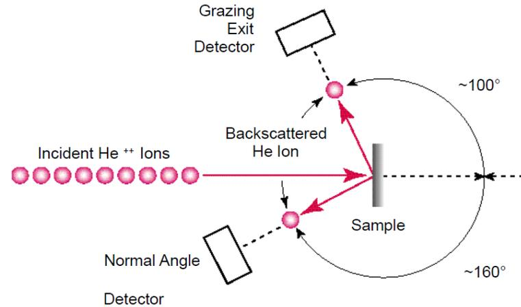
Grazing angle detector improves depth resolution for thin film layer
