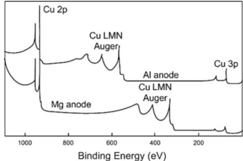
Cu XP spectra illustrating the shift in Auger peak positions with change from Mg to Al anodes in the x-ray source ( Auger is dependent on the photon energy)
