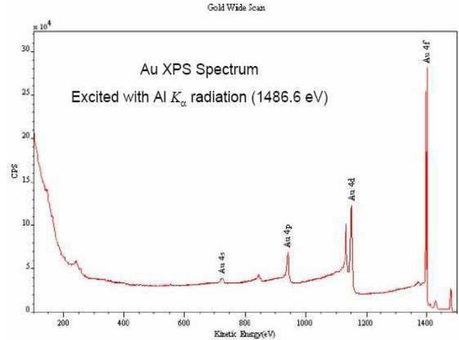
atoms have valence and core electrons: Core-level Binding energies provide unique signature of elements.
