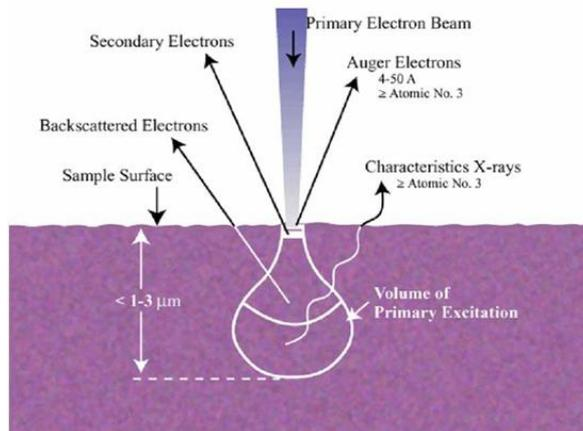
**Backscattered electrons (BSEs):** are primary e<sup>-</sup>s leaving the specimen after a few large angle elastic scattering events
