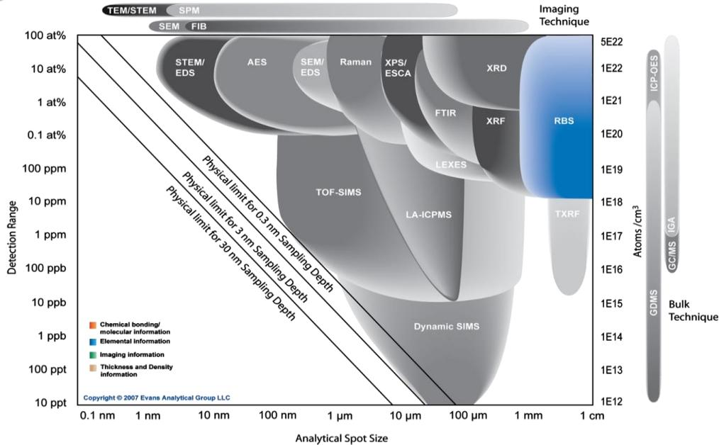
RBS accurately measures the composition and depth profile of thin films, including hydrogen
