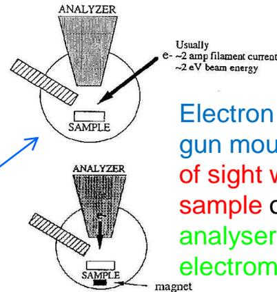
Electron flood gun mounted line of sight with sample or in analyser axis + electromagnet
