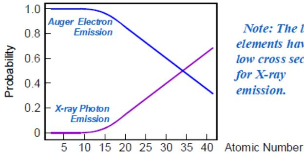
*Note: The light elements have a low cross section for X-ray emission.*
