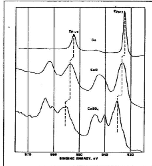
Arises when a core electron is removed by photoionization. There is a sudden change in the effective charge due to loss of shielding electrons.
