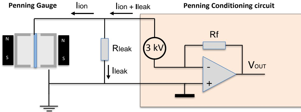
$$V_{OUT} = R_f \cdot (I_{ion} + I_{leak})$$
