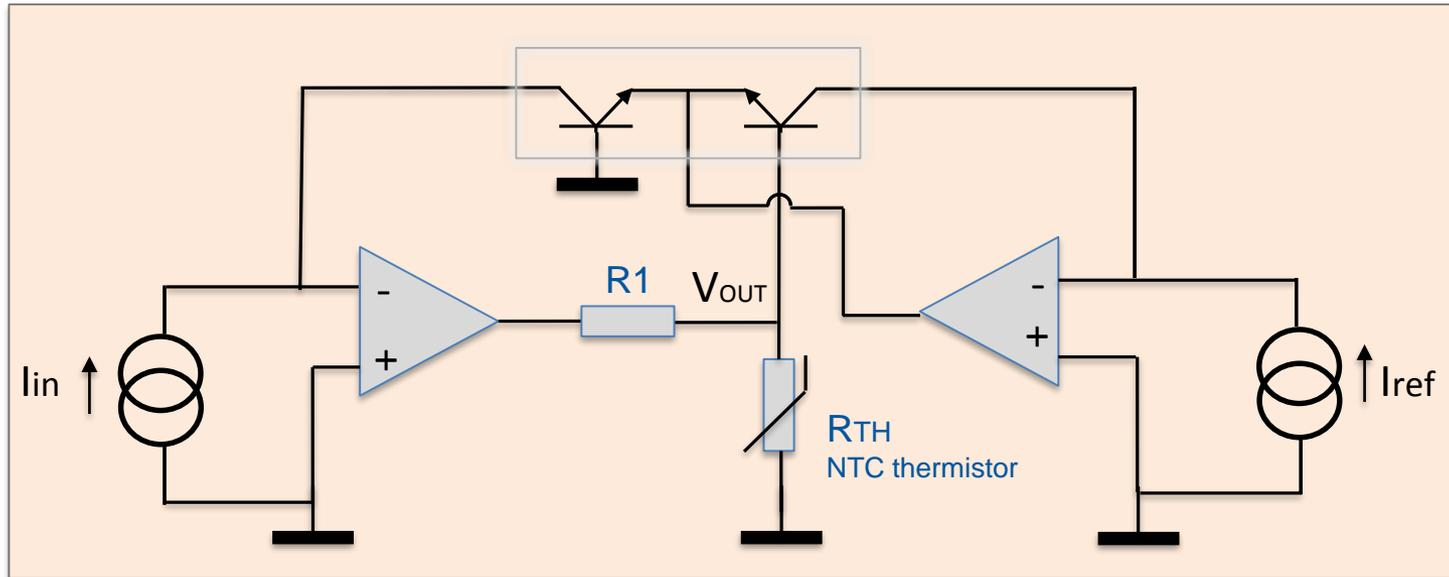
$$V_{OUT} = \left(1 + \frac{R_1}{R_{TH}}\right) \frac{kT}{q \cdot \log_{10} e} \cdot \log_{10} \left(\frac{I_{in}}{I_{ref}}\right)$$
