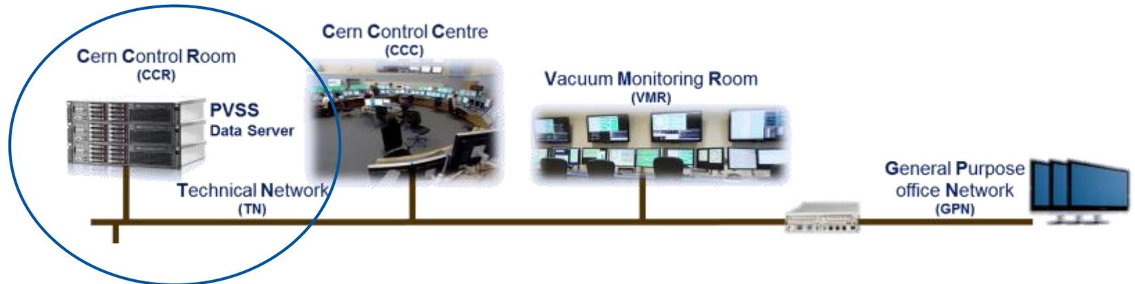
CERN's vacuum SCADA is based on **WinCC-OA** (Open Architecture) from Siemens (former PVSS from ETM).
