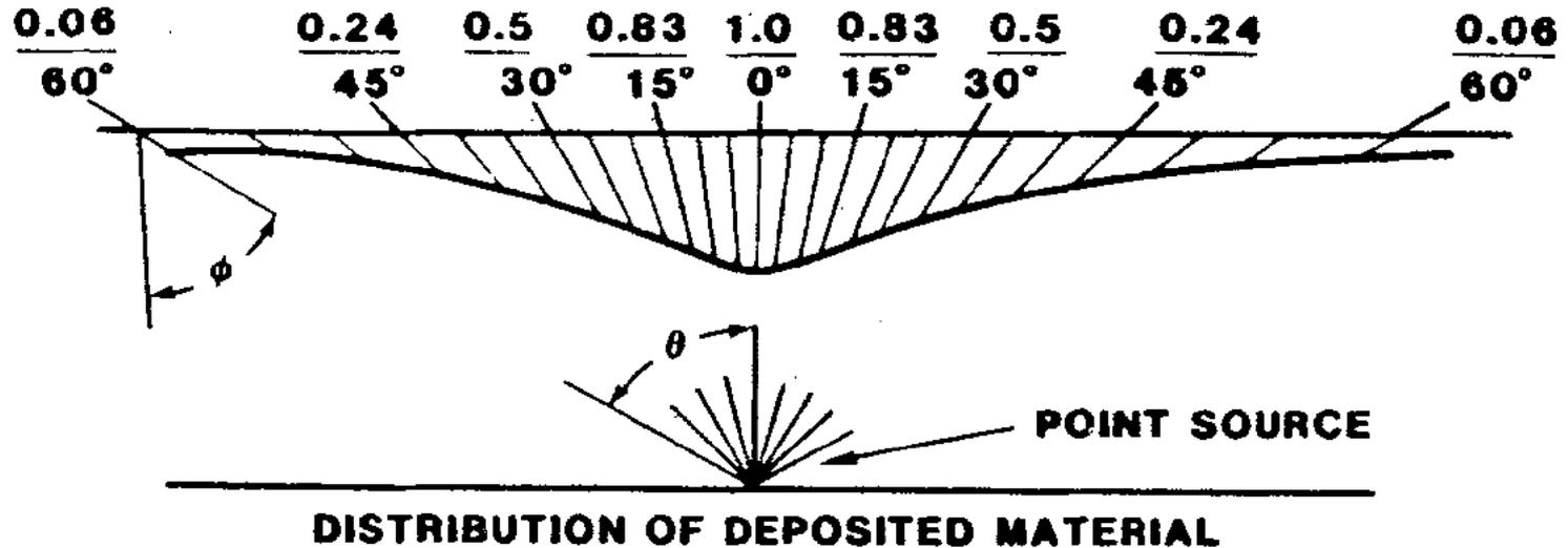
Fig. 4. Cosine distribution of vapor from a point source.
