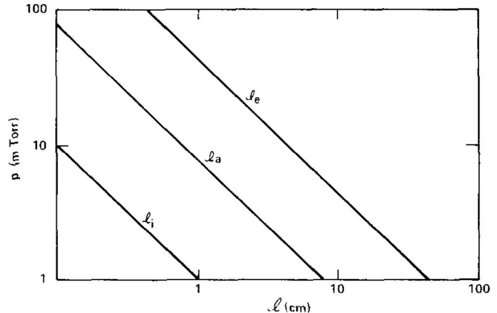
FIG. 2. Mean free paths for atoms,  $l_a$ , electrons,  $l_e$ , and ions,  $l_i$ , as a function of pressure in the argon glow discharge, calculated from kinetic gas theory.
