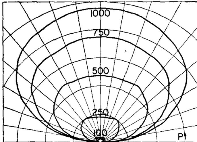
FIG. 3. Polar diagram of material sputtered from Pt by normally incident  $\text{Hg}^+$  ions of 100 to 1000 eV energy.
