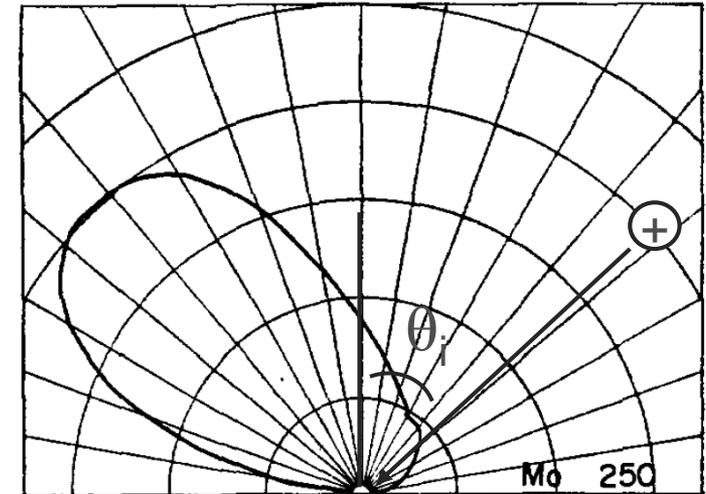
FIG. 9. Polar diagram of material sputtered from Mo by obliquely incident  $\text{Hg}^+$  ions of 250 eV energy. One edge of a Mo strip by obliquely incident  $\text{Hg}^+$  ions of 250 eV.
