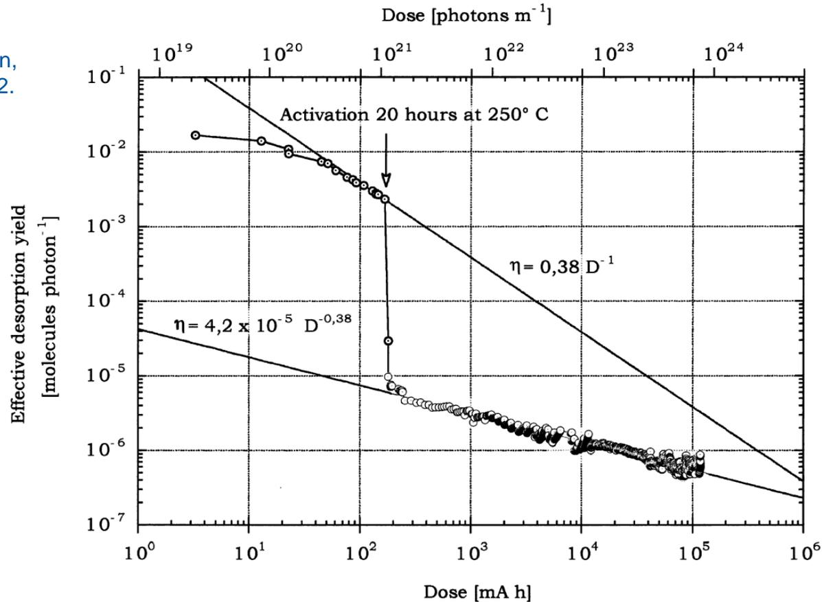
Fig. 2. Total molecular desorption yield  $\eta$  ( $N_2$  equivalent) of the Ti-Zr-V coated stainless-steel chamber as a function of the accumulated dose before and after activation.
