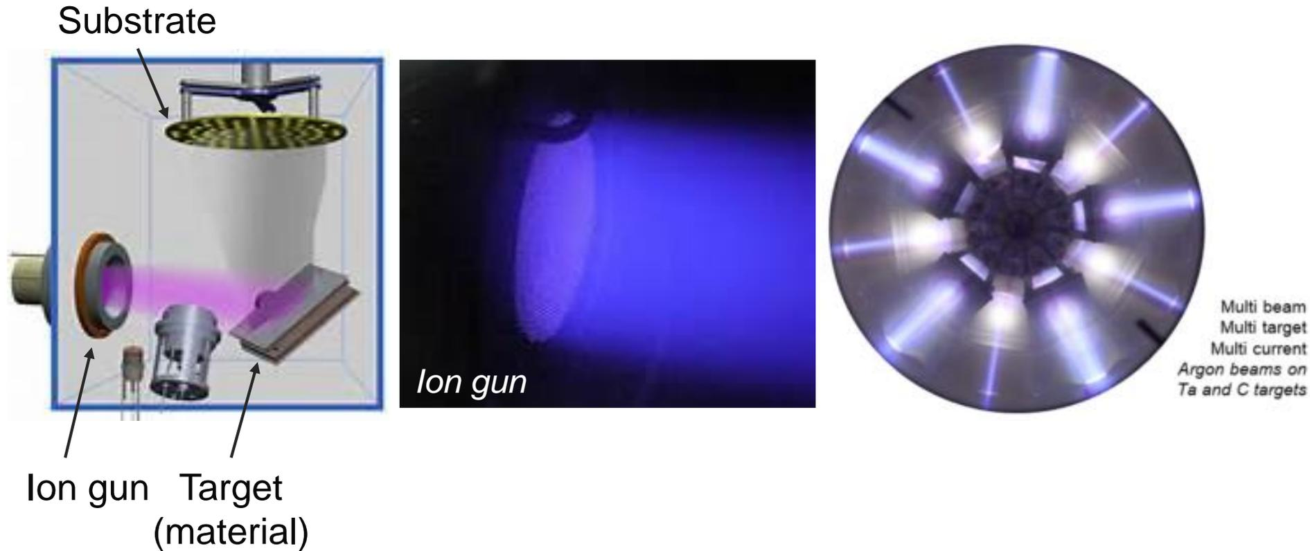
Not convenient to coat tubes or large area substrates!
