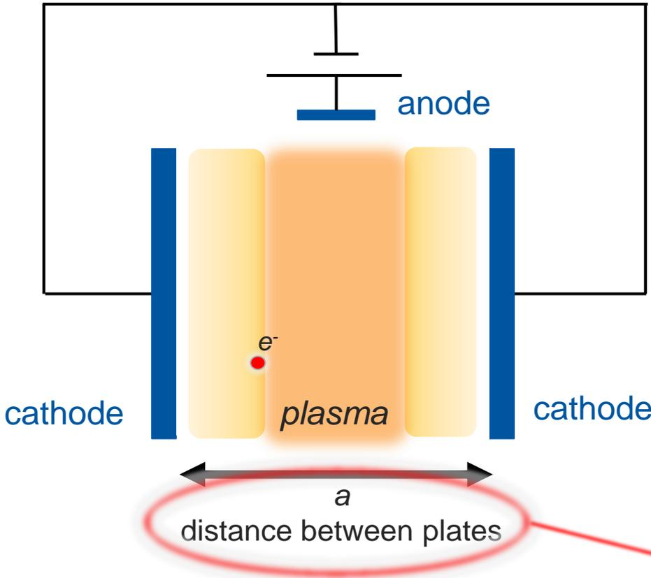
*Pendel electrons -> increase ionization efficiency*
