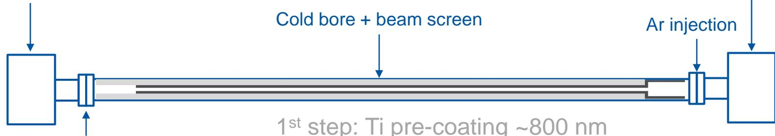
1<sup>st</sup> step: Ti pre-coating ~800 nm
